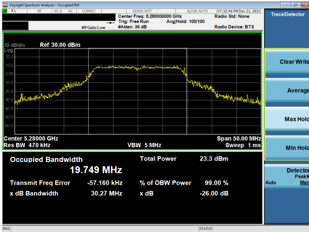
Plot 7-9. 26dB Bandwidth Plot MIMO ANT1 (20MHz BW 802.11n (UNII Band 2A) – Ch. 56)
