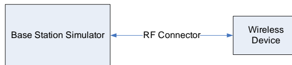
Figure 9-3 Power Measurement Setup
