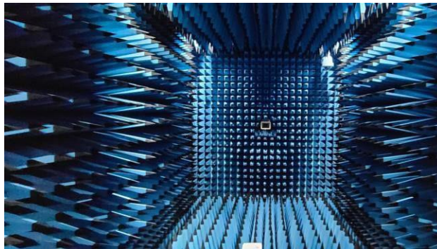
Figure 2: Geometry of Anechoic Chamber for Radiation patterns.
