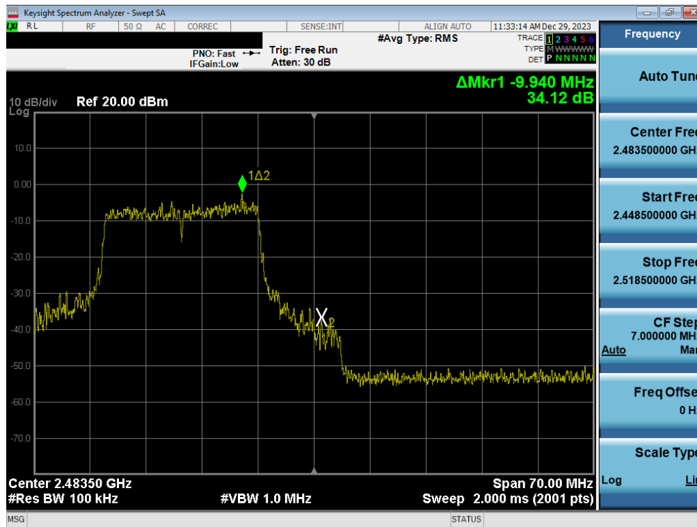
Plot 7-32. Band Edge Plot MIMO ANT1 (802.11ax OFDMA – 242 Tones – Ch. 13)
