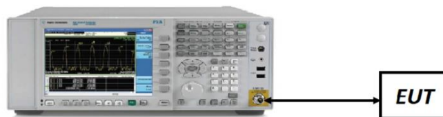
Figure 7-1. Test Instrument & Measurement Setup
