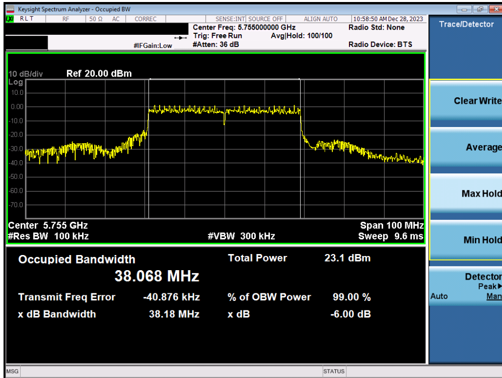
Plot 7-47. 6dB Bandwidth Plot MIMO ANT2 (40MHz BW 802.11ax – 484 Tones (UNII Band 3) – Ch. 151)
