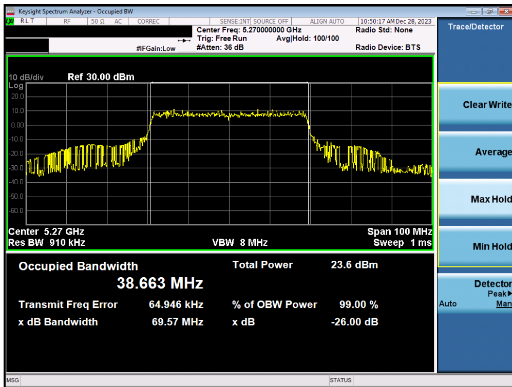
Plot 7-32. 26dB Bandwidth Plot MIMO ANT2 (40MHz BW 802.11ax – 484 Tones (UNII Band 2A) – Ch. 54)
