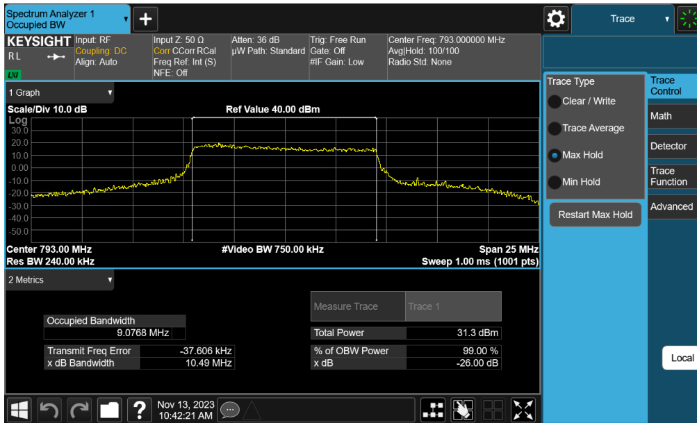
Plot 7-2. Occupied Bandwidth Plot (LTE Band 14 - 10MHz 16-QAM - Full RB)
