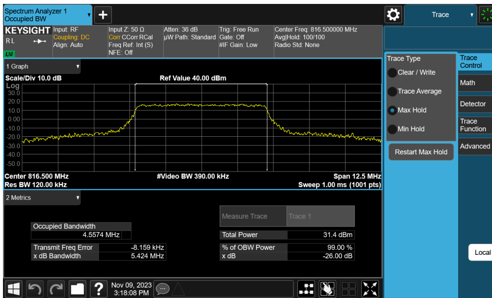
Plot 7-10. Occupied Bandwidth Plot (LTE Band 26 - 5MHz 16-QAM - Full RB)
