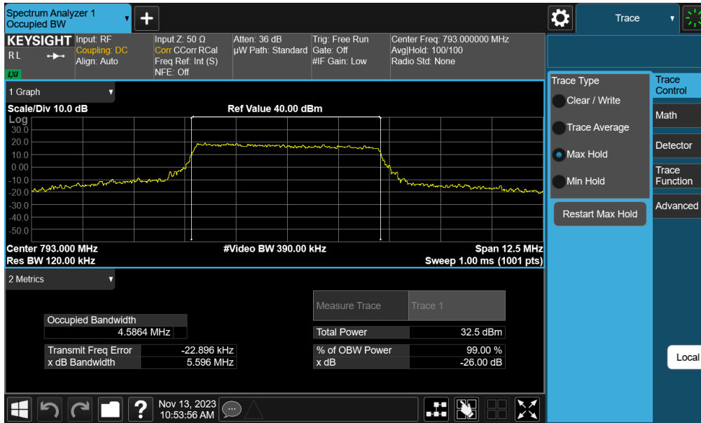
Plot 7-3. Occupied Bandwidth Plot (LTE Band 14 - 5MHz QPSK - Full RB)
