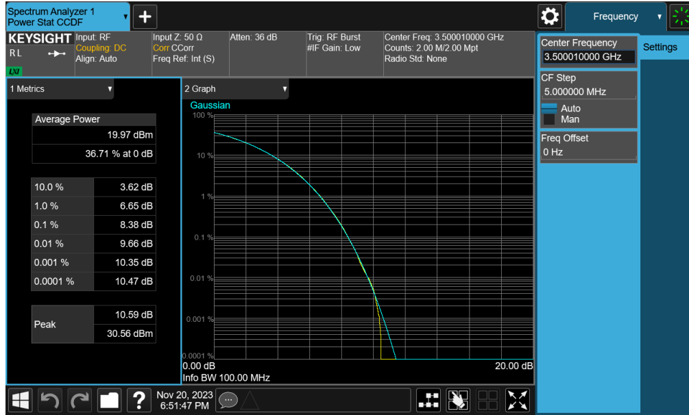
Plot 7-118. PAR Plot (NR Band n77/78 DoD - 100MHz CP-OFDM 256-QAM - Full RB - Ant 1)
