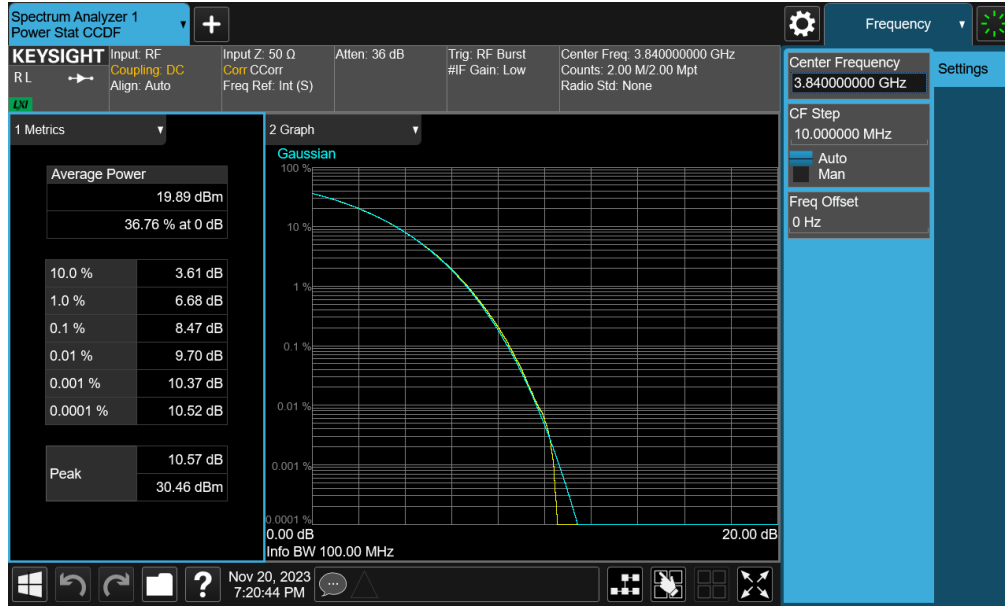
Plot 7-115. PAR Plot (NR Band n77/78 - 100MHz CP-OFDM 256-QAM - Full RB - Ant 1)
