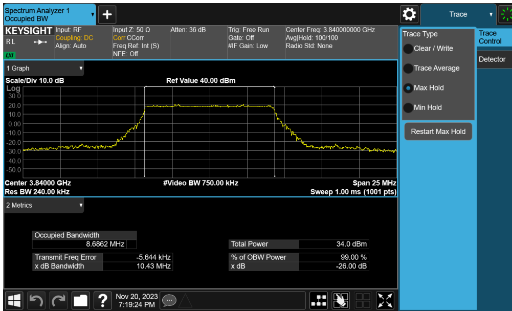
Plot 7-34. Occupied Bandwidth Plot (NR Band n77/78 - 10MHz π/2 BPSK - Full RB - Ant 1)
