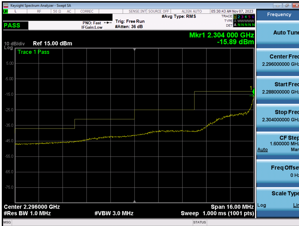
Plot 7-191. Extended Lower Band Edge Plot (LTE Band 30 - 5MHz QPSK – Full RB - Ant2)
