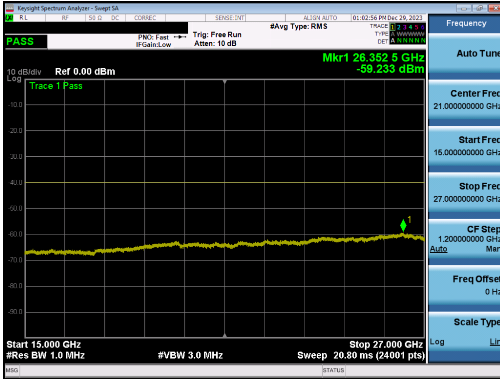
Plot 7-159. Conducted Spurious Plot (LTE Band 30 - 10MHz QPSK - RB Size 1, RB Offset 0 - Ant2)
