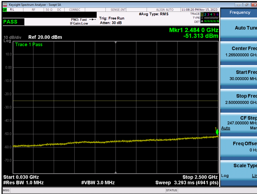
Plot 7-138. Conducted Spurious Plot (LTE Band 7 - 20MHz QPSK - RB Size 1, RB Offset 0 - High Channel - Ant1)
