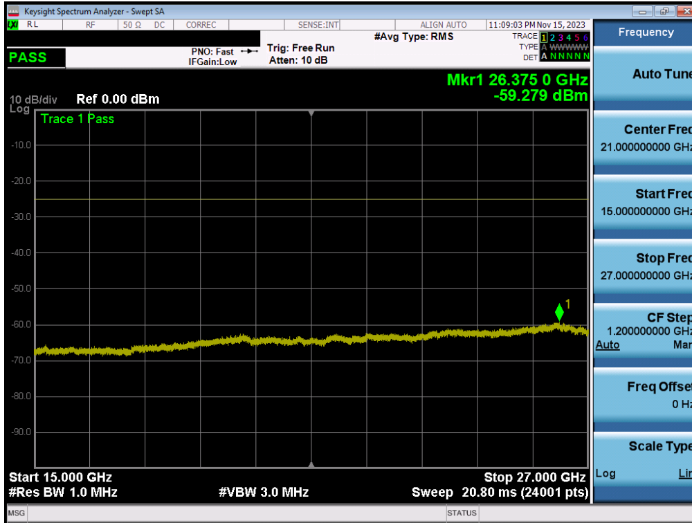
Plot 7-140. Conducted Spurious Plot (LTE Band 7 - 20MHz QPSK - RB Size 1, RB Offset 0 - High Channel - Ant1)
