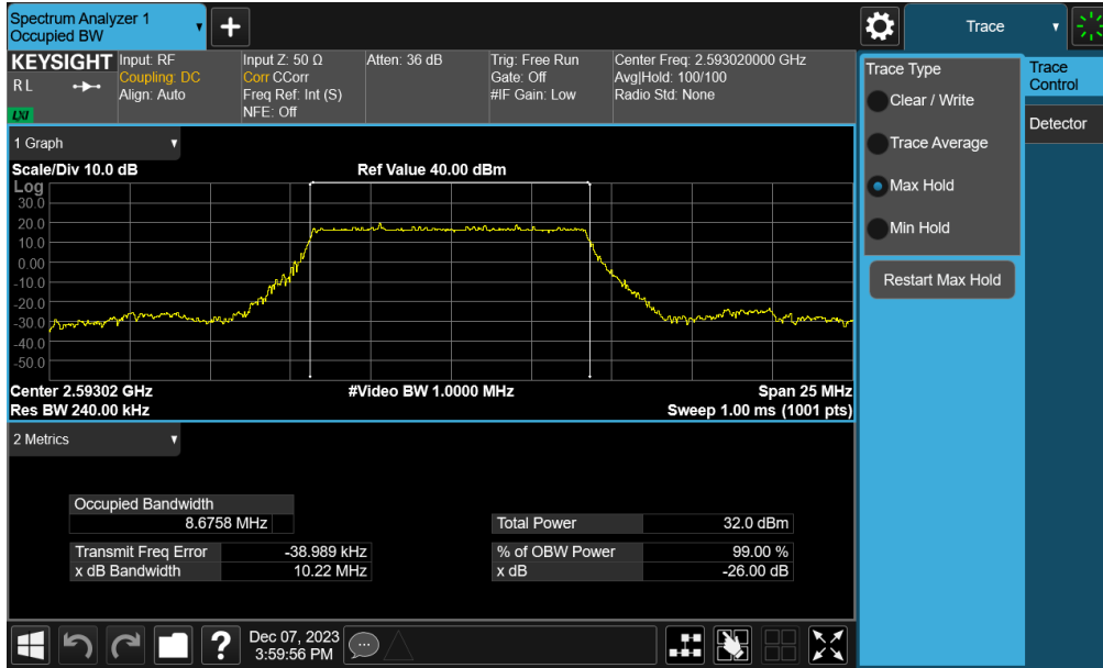
Plot 7-132. Occupied Bandwidth Plot (NR Band n41- 10MHz \pi/2 BPSK - Full RB Configuration – Ant2)
