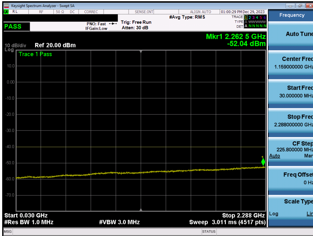
Plot 7-157. Conducted Spurious Plot (LTE Band 30 - 10MHz QPSK - RB Size 1, RB Offset 0 - Ant2)
