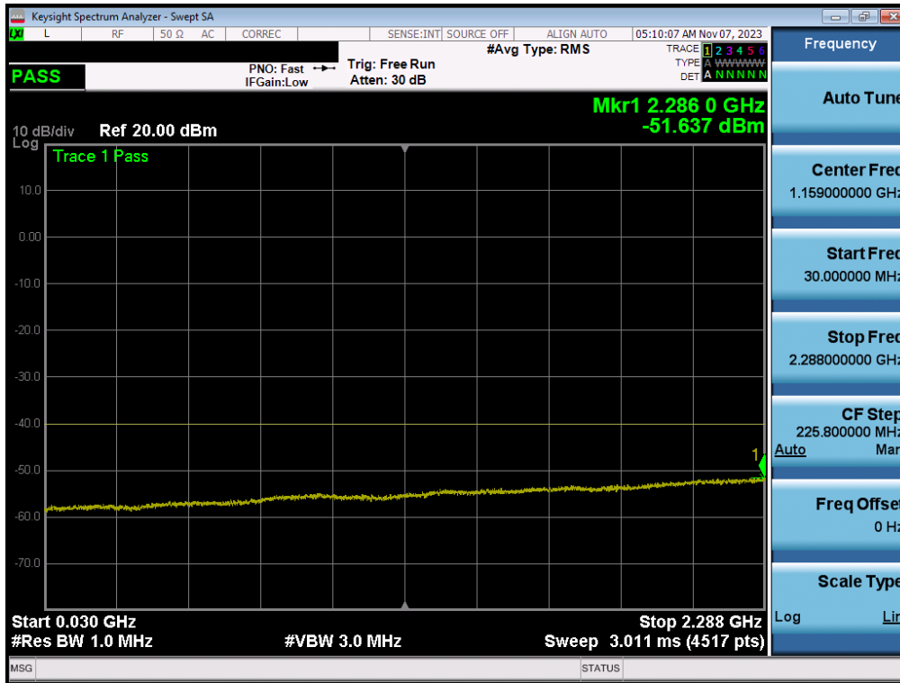
Plot 7-135. Conducted Spurious Plot (LTE Band 30 - 10MHz QPSK - RB Size 1, RB Offset 0 - Ant1)
