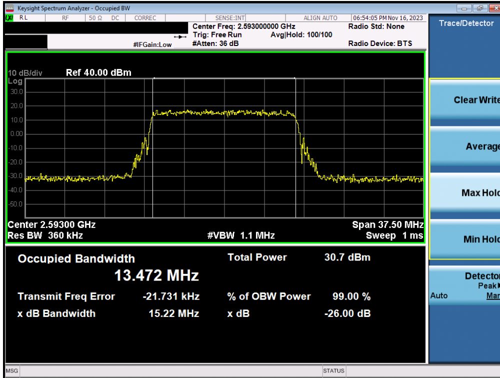
Plot 7-23. Occupied Bandwidth Plot (LTE Band 38 - 15MHz QPSK - Full RB - Ant1)
