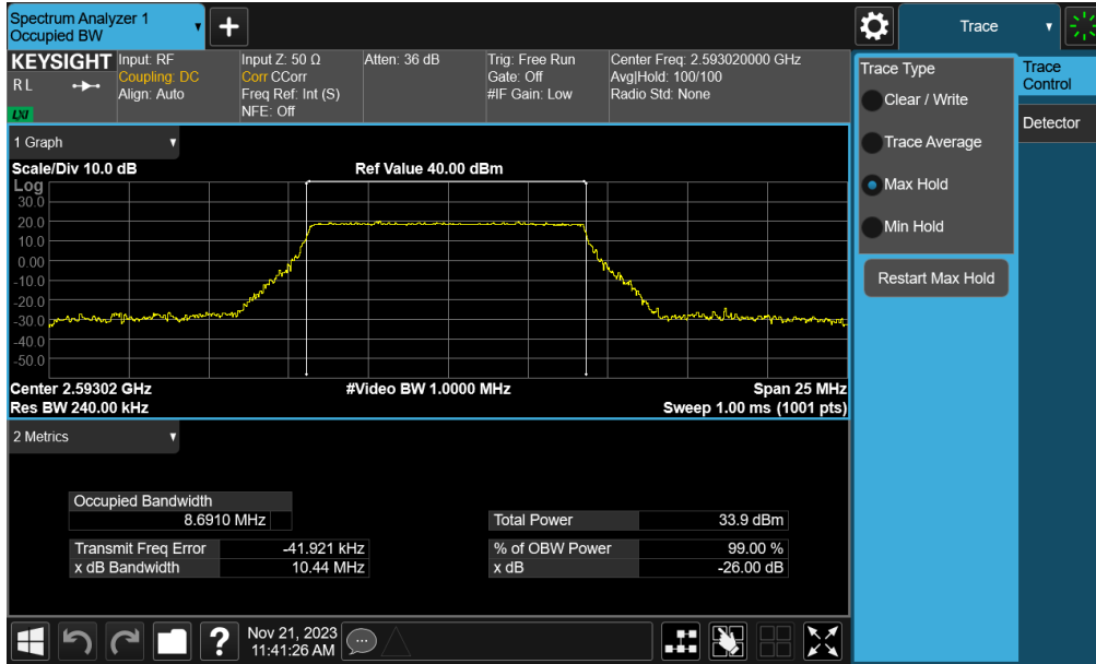
Plot 7-65. Occupied Bandwidth Plot (NR Band n41 - 10MHz \pi/2 BPSK - Full RB Configuration - Ant1)
