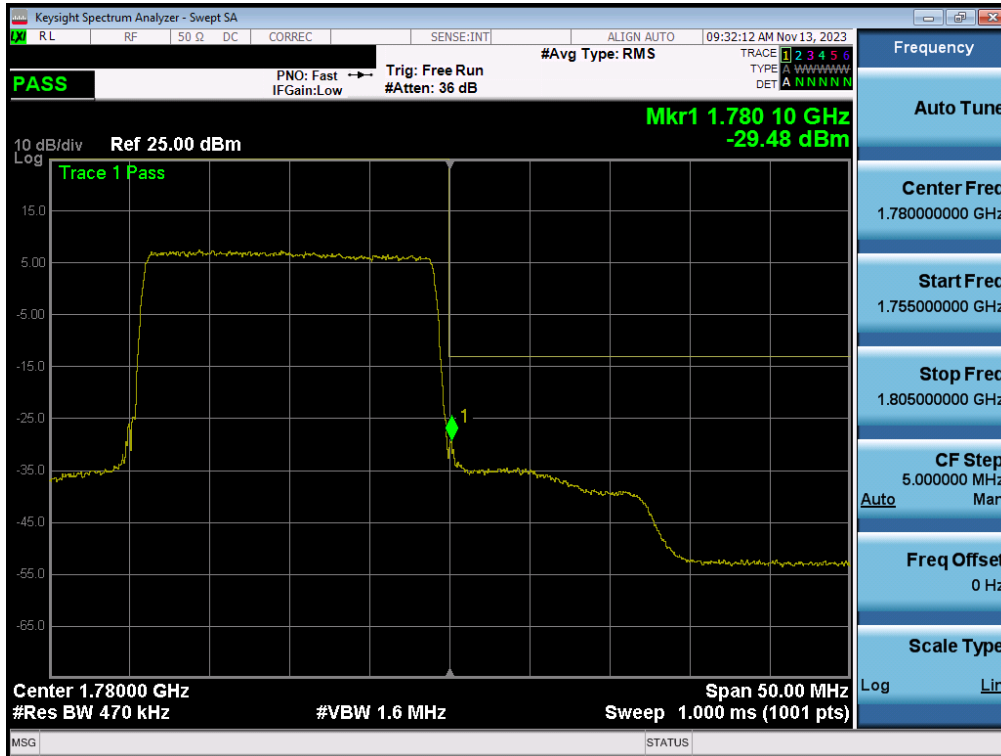
Plot 7-177. Upper Band Edge Plot (LTE Band 66 - 20MHz QPSK - Full RB - ANT2)
