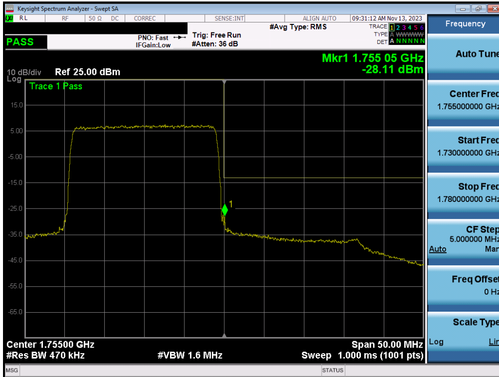
Plot 7-175. Upper Band Edge Plot (LTE Band 4 - 20MHz QPSK – Full RB - ANT2)
