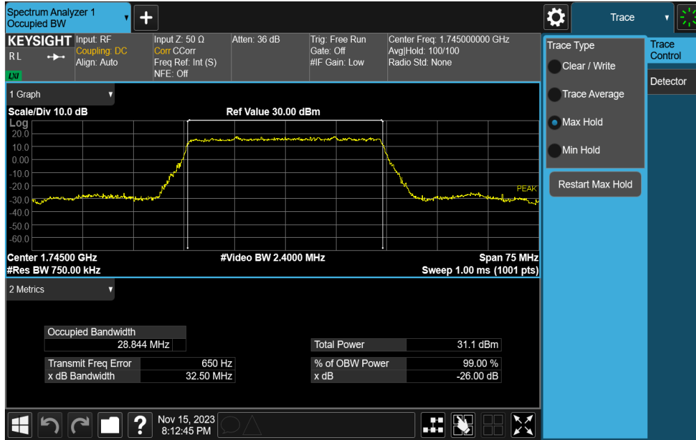
Plot 7-97. Occupied Bandwidth Plot (NR Band n66 - 30.0MHz DFT-s-OFDM BPSK - Full RB – ANT2)
