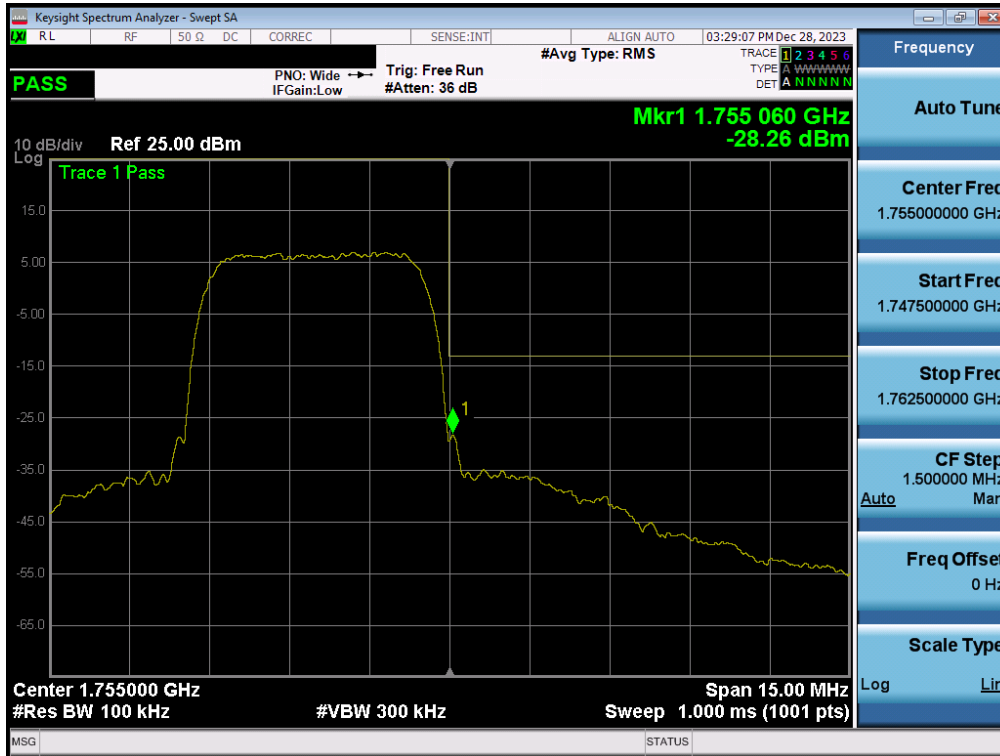
Plot 7-147. Upper Band Edge Plot (WCDMA AWS – Ch. 1513 – ANT1)
