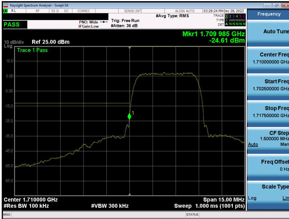
Plot 7-145. Lower Band Edge Plot (WCDMA AWS – Ch. 1312 – ANT1)
