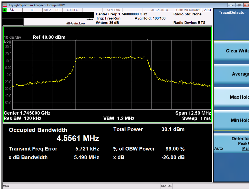
Plot 7-86. Occupied Bandwidth Plot (LTE Band 66/4 - 5MHz 16-QAM - Full RB - ANT2)
