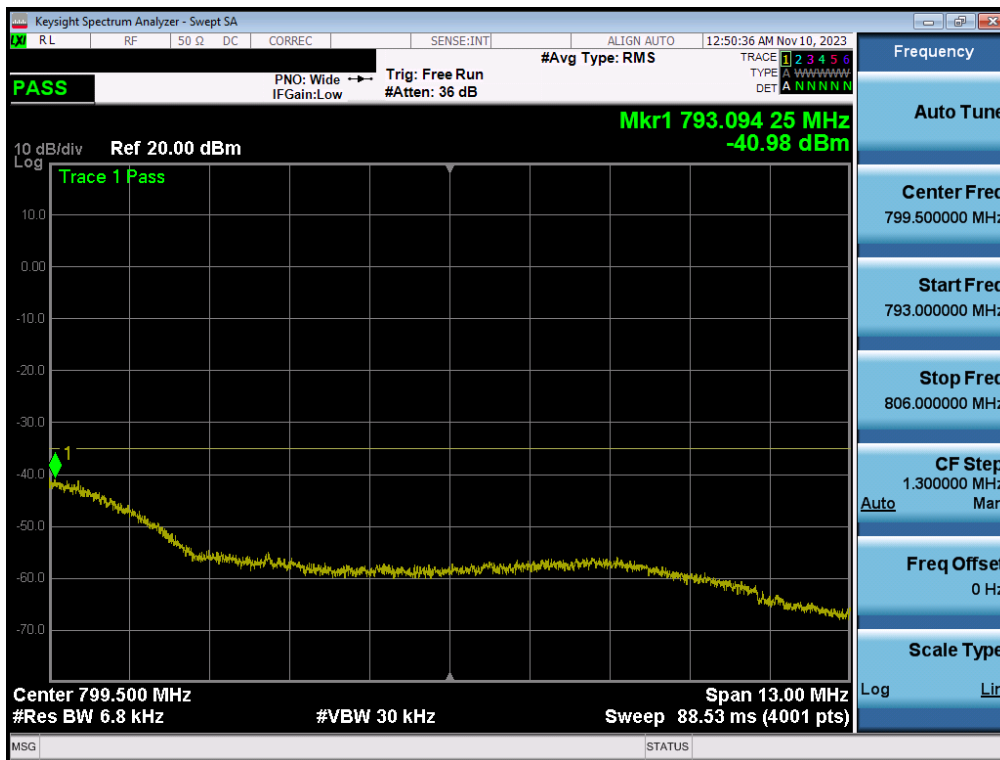
Plot 7-156. Upper Emission Mask Plot (LTE Band 13 - 10MHz QPSK – Full RB - ANT1)
