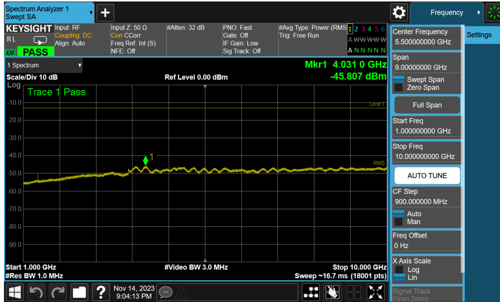
Plot 7-129. Conducted Spurious Plot (NR Band n71 - 20.0MHz - 1 RB - Mid Channel - ANT1)
