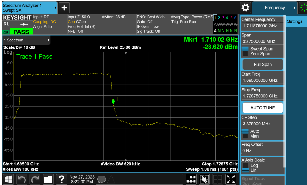
Plot 7-167. Upper Band Edge Plot (NR Band n70 – 10.0MHz - Full RB - ANT1)
