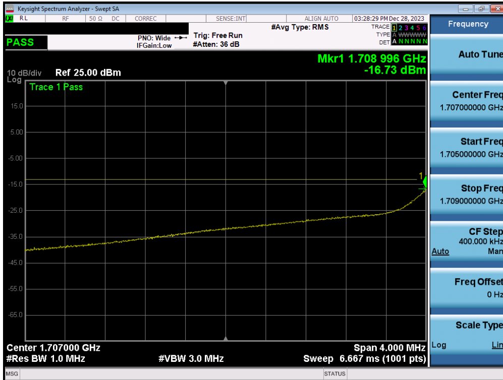
Plot 7-146. Lower Extended Band Edge Plot (WCDMA AWS – Ch. 1312 – ANT1)
