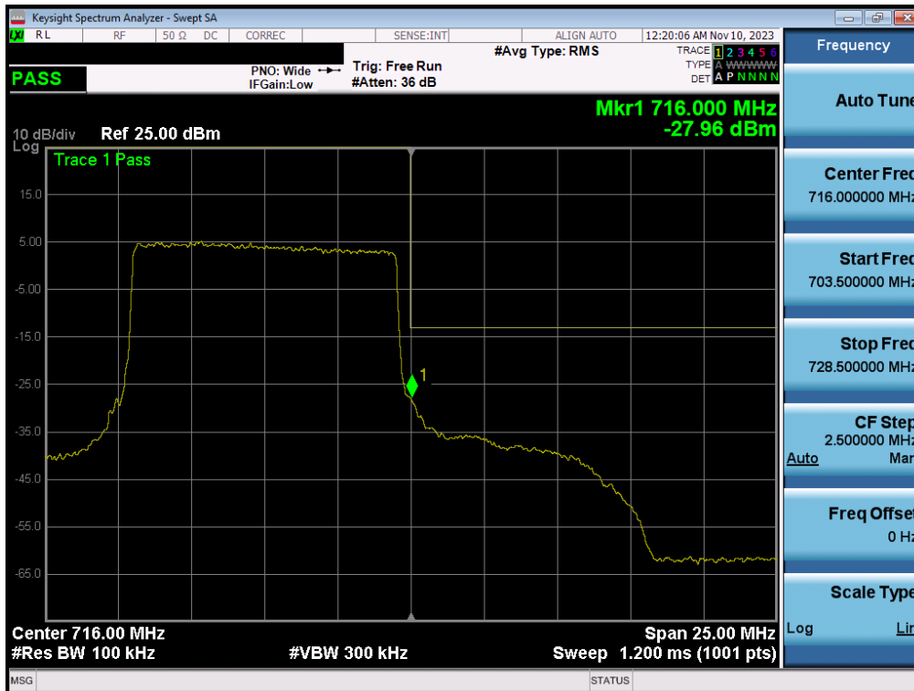
Plot 7-152. Upper Band Edge Plot (LTE Band 12 – 10MHz QPSK – Full RB - ANT1)
