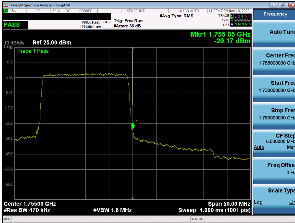
Plot 7-159. Upper Band Edge Plot (LTE Band 4 - 20MHz QPSK – Full RB - ANT1)
