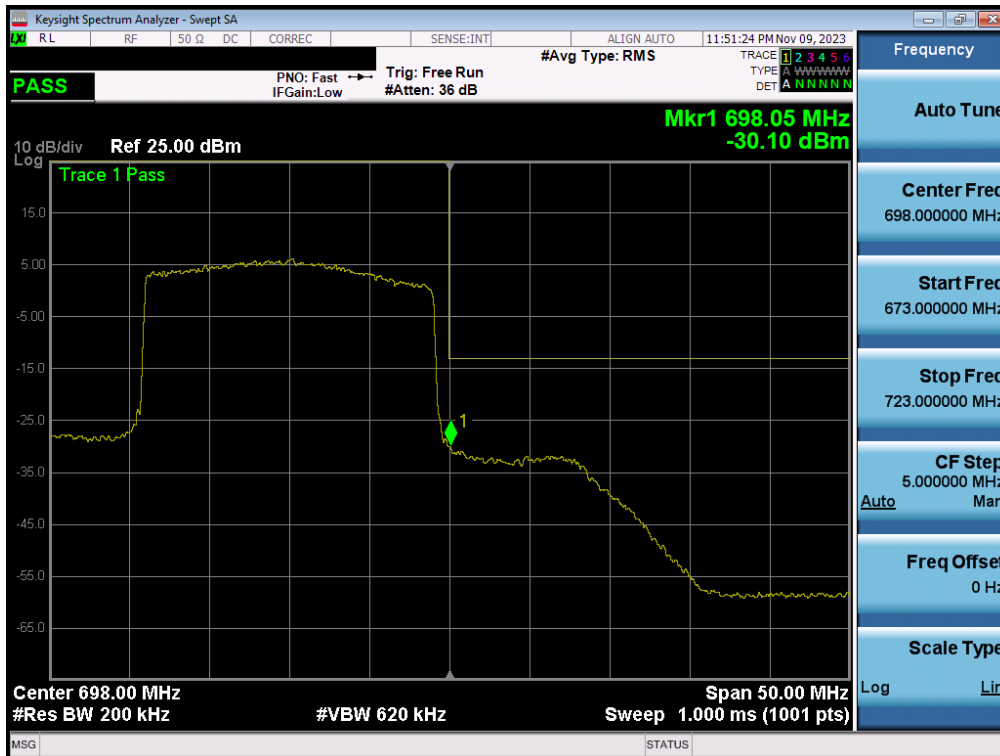
Plot 7-150. Upper Band Edge Plot (LTE Band 71 – 20MHz QPSK – Full RB - ANT1)
