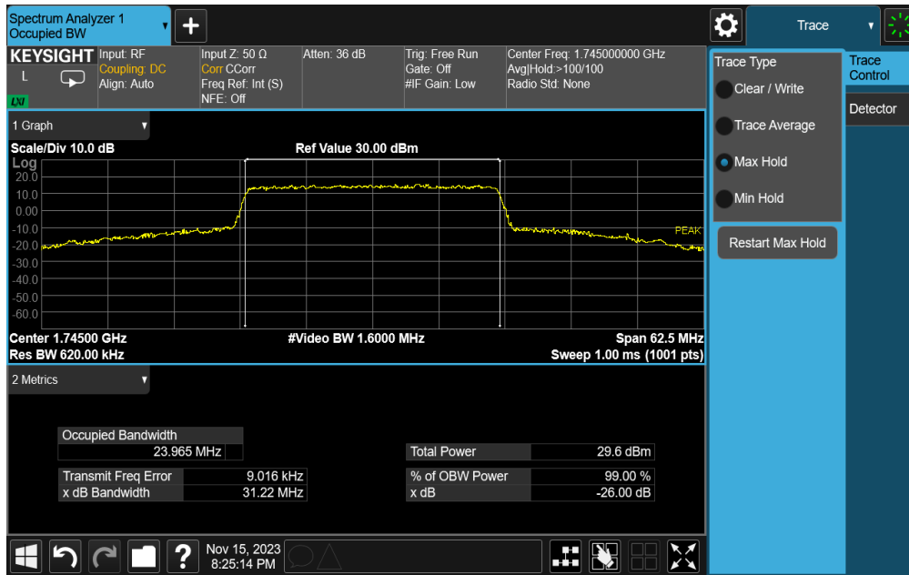
Plot 7-102. Occupied Bandwidth Plot (NR Band n66 - 25.0MHz CP-OFDM 16QAM - Full RB – ANT2)
