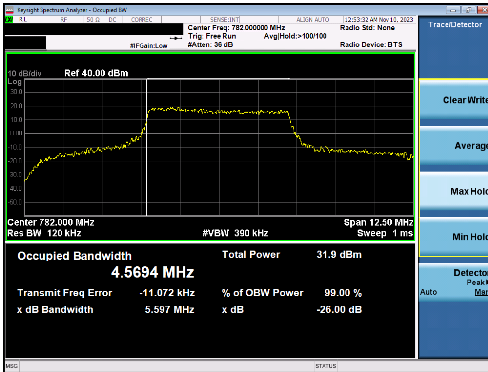
Plot 7-21. Occupied Bandwidth Plot (LTE Band 13 - 5MHz 16-QAM - Full RB – ANT1)
