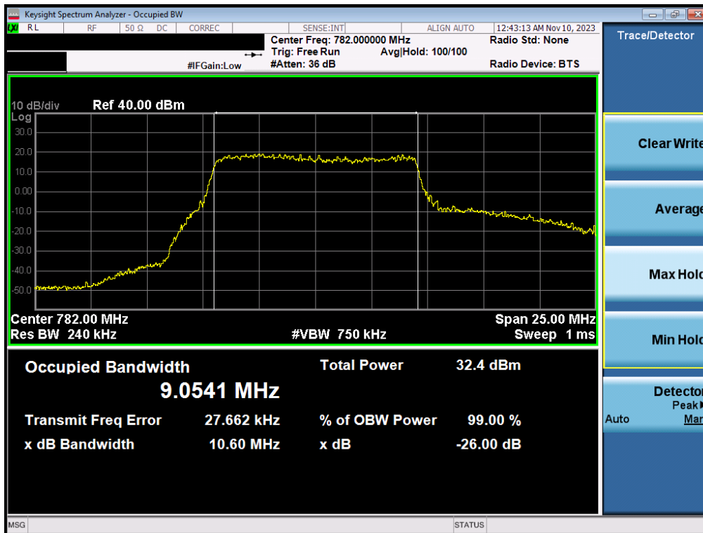
Plot 7-19. Occupied Bandwidth Plot (LTE Band 13 - 10MHz 16-QAM - Full RB – ANT1)
