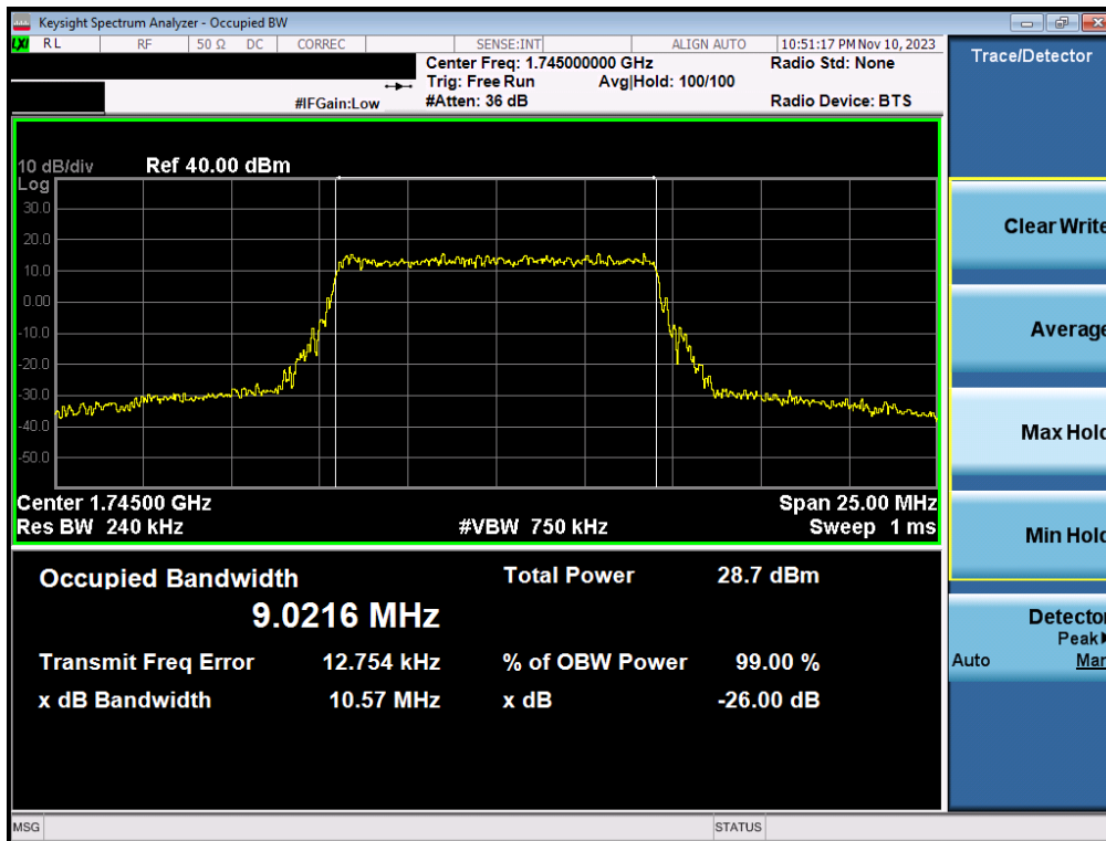
Plot 7-48. Occupied Bandwidth Plot (LTE Band 66/4 - 10MHz 16-QAM - Full RB - ANT1)
