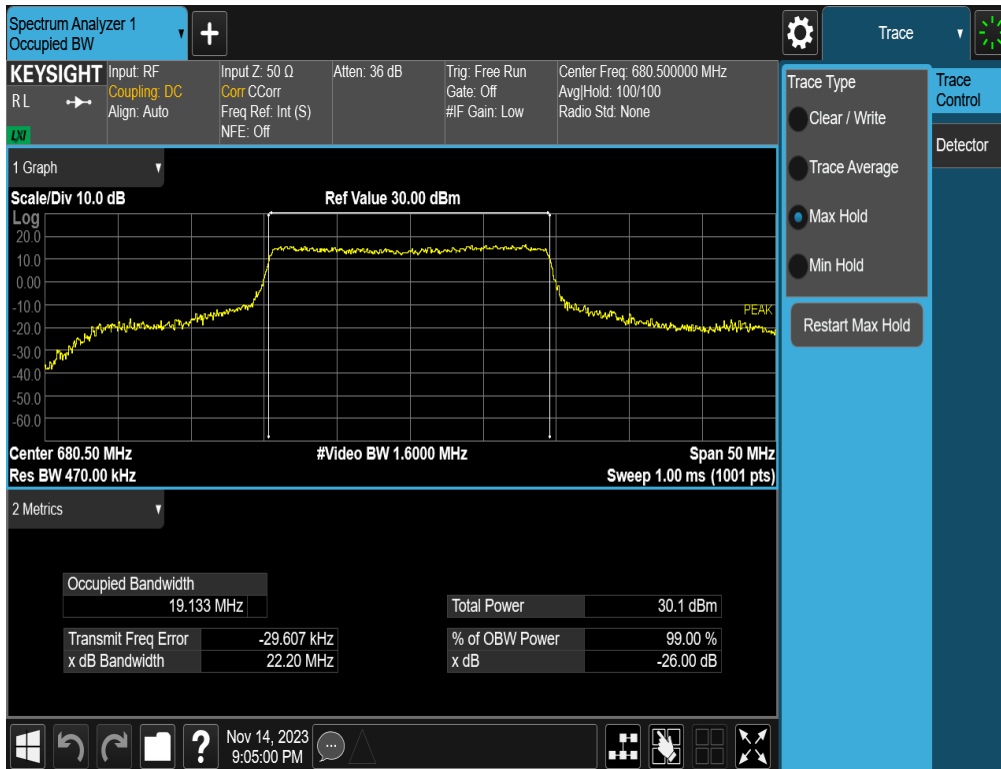
Plot 7-23. Occupied Bandwidth Plot (NR Band n71 - 20MHz CP-OFDM QPSK - Full RB – ANT1)
