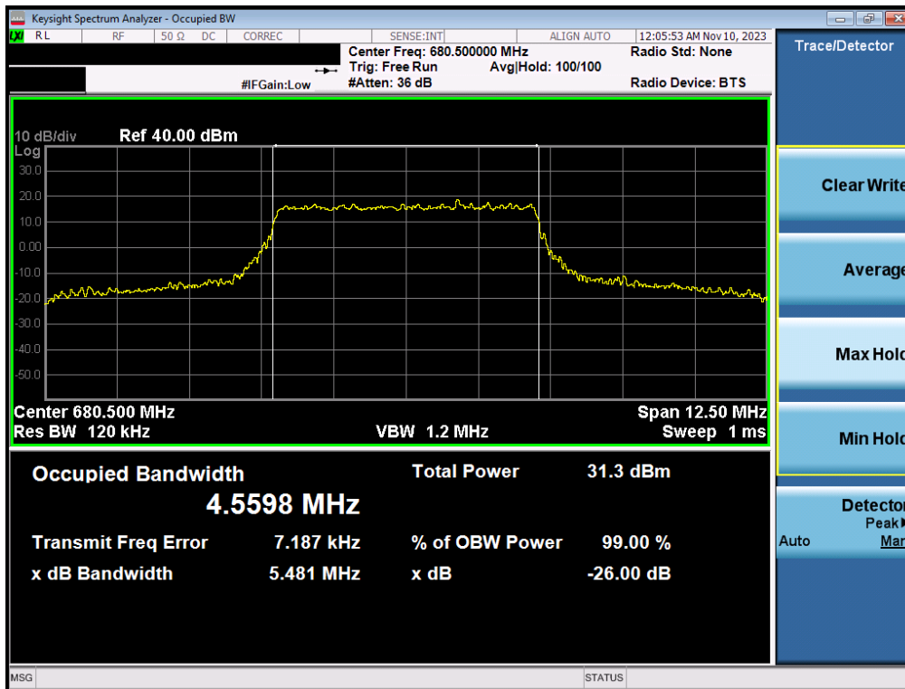
Plot 7-9. Occupied Bandwidth Plot (LTE Band 71 - 5MHz 16-QAM - Full RB - ANT1)
