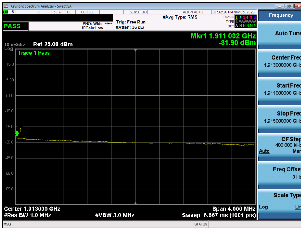
Plot 7-35. Extended Upper Band Edge Plot (LTE Band 2 - 20MHz QPSK – Full RB - Ant1)
