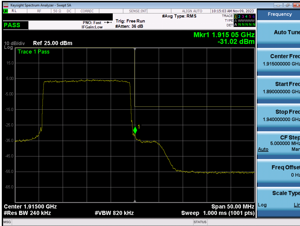
Plot 7-42. Upper Band Edge Plot (LTE Band 25 - 20MHz QPSK – Full RB - Ant2)
