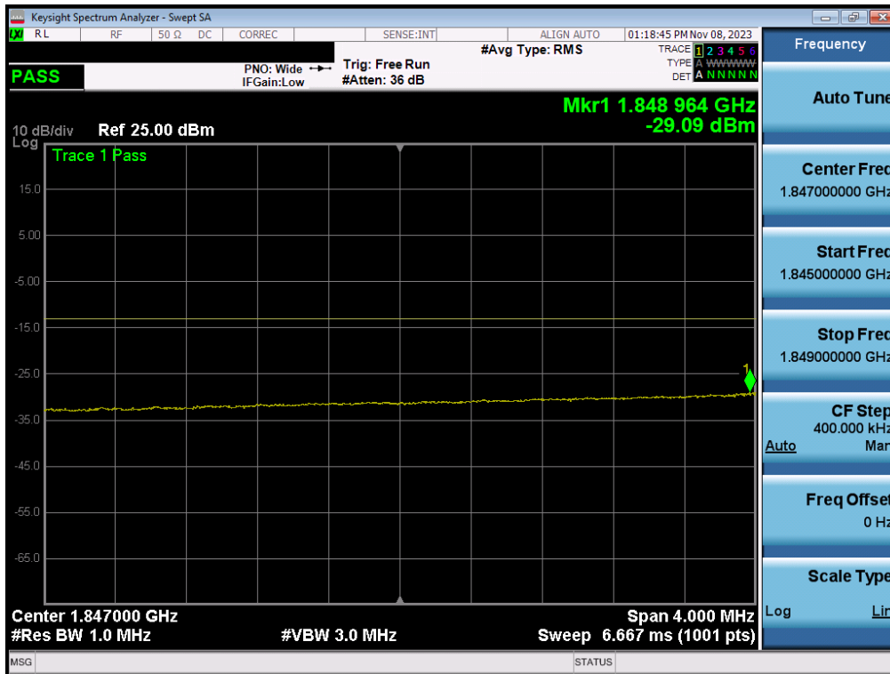
Plot 7-33. Extended Lower Band Edge Plot (LTE Band 25/2 - 20MHz QPSK – Full RB - Ant1)
