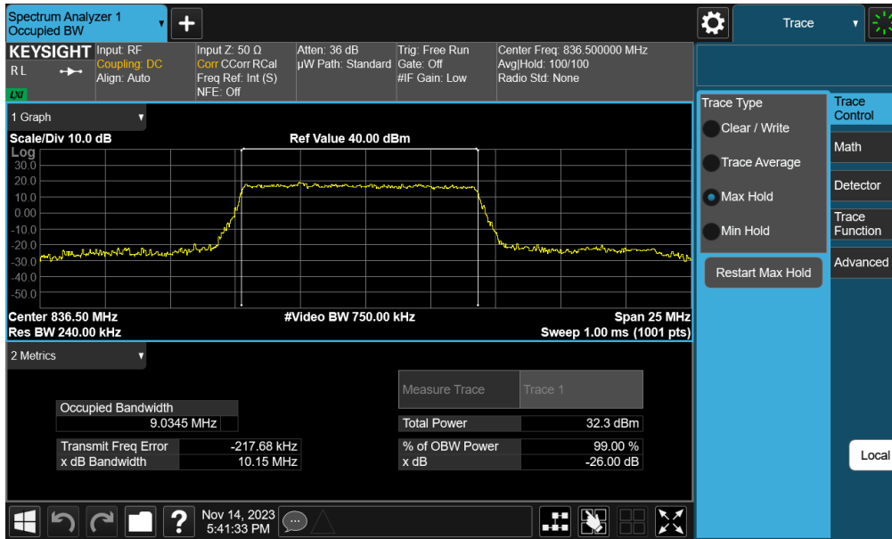
Plot 7-17. Occupied Bandwidth Plot (NR Band n5 - 10MHz \pi/2 BPSK - Full RB)
