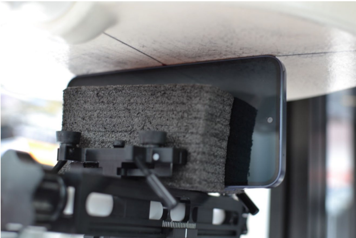
SAR Test Setup Photo 16 – Phablet, Left Edge at 0mm
