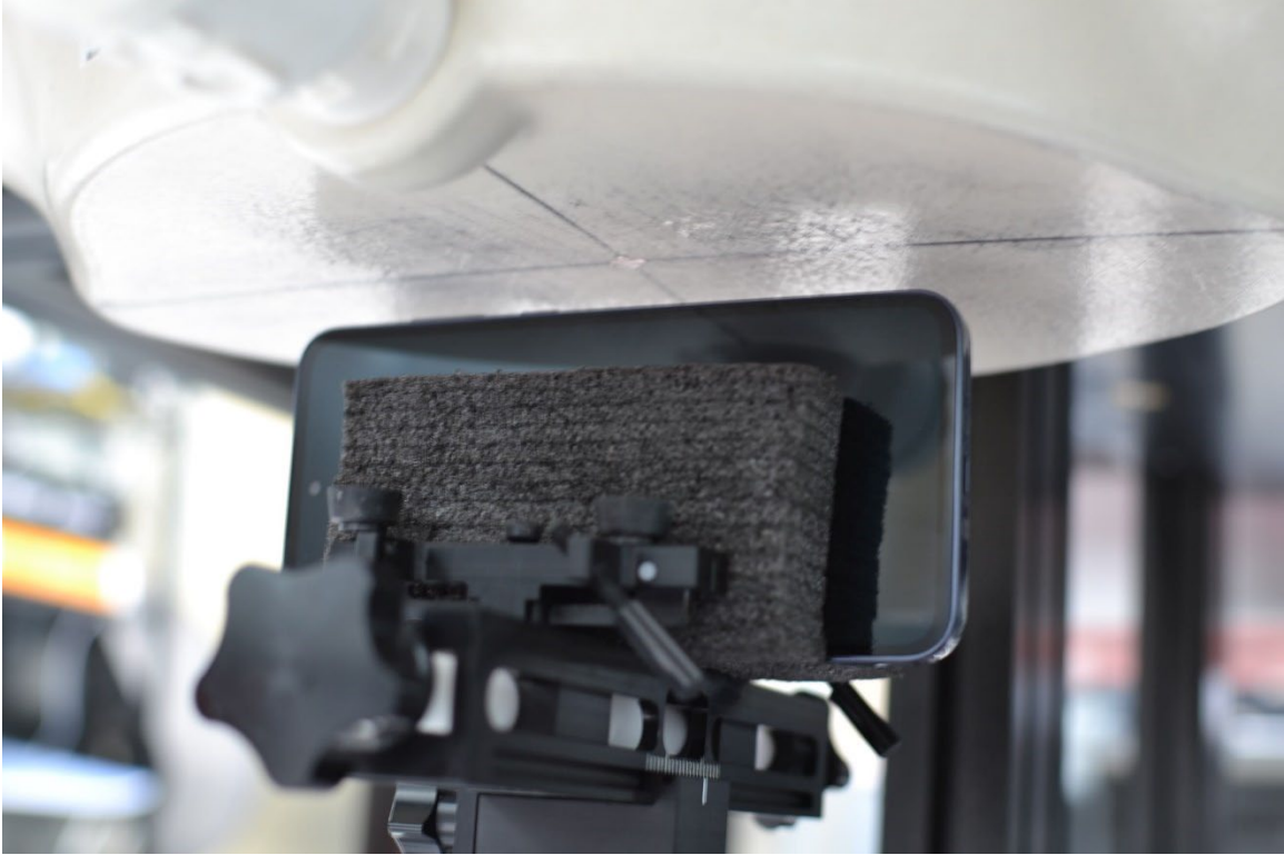
SAR Test Setup Photo 13 – Hotspot, Right Edge at 10mm
