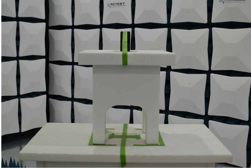
Figure 3. Test Setup – Z Position – 1GHz-18GHz
