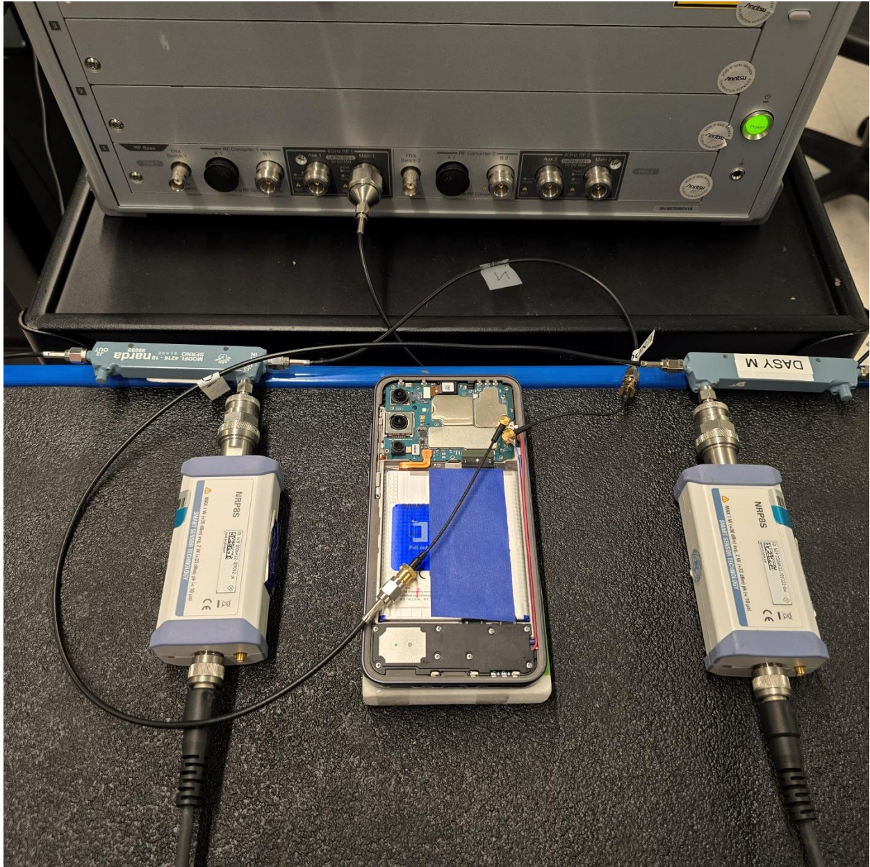
Test Setup Photo 4 - Conducted Test Setup (Figure 6-1c)
