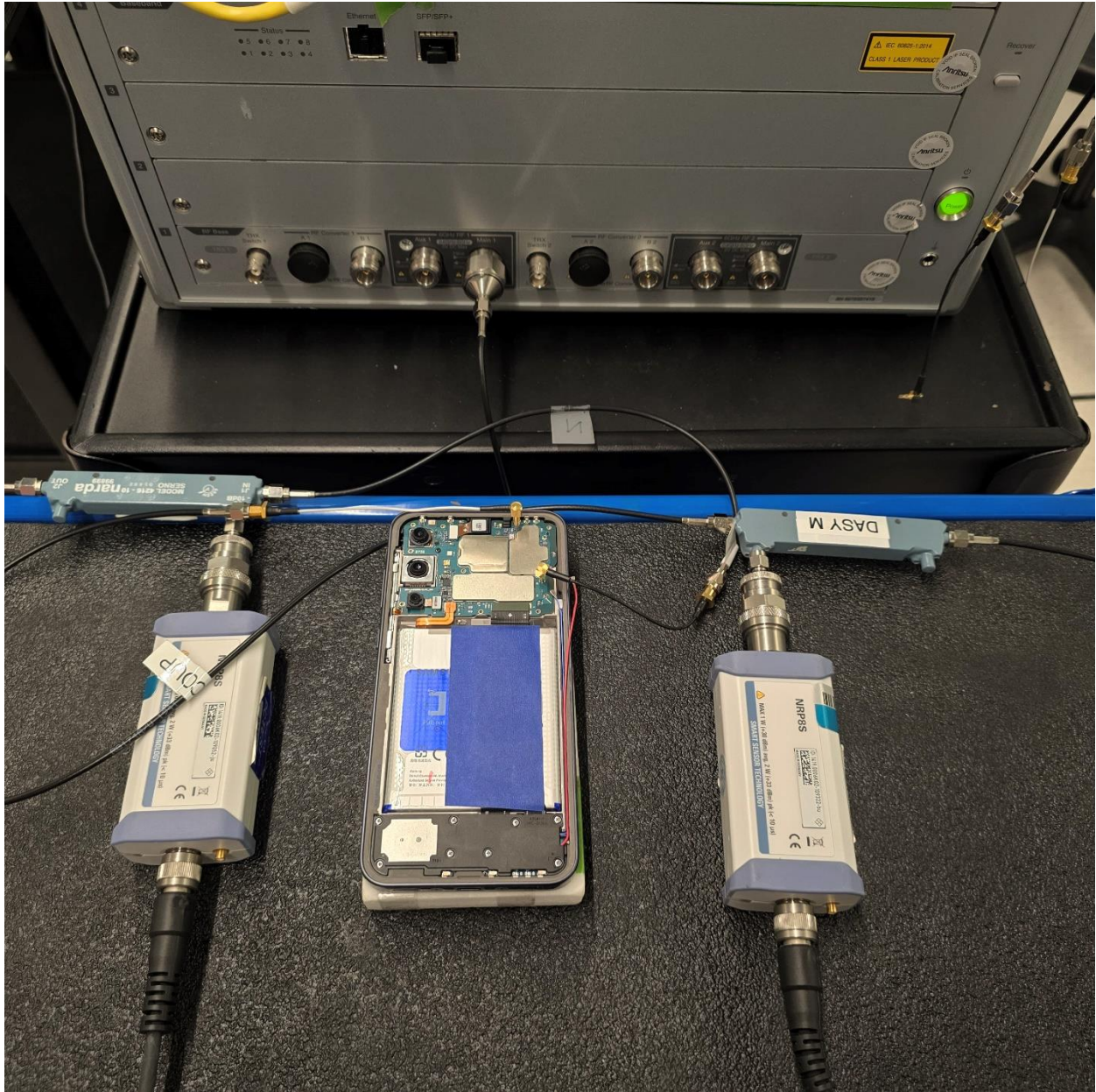
Test Setup Photo 7 – Conducted Test Setup (Figure 6-1c)
