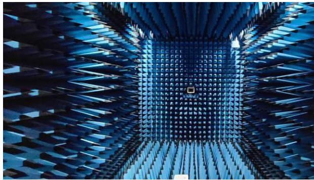
Figure 2: Geometry of Anechoic Chamber for Radiation patterns.
