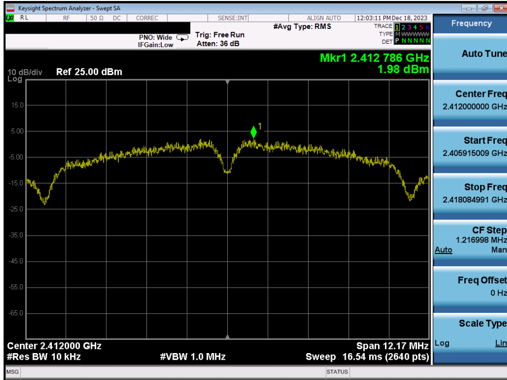
Plot 7-25. Power Spectral Density Plot (802.11b – Ch. 1) – MIMO ANT1
