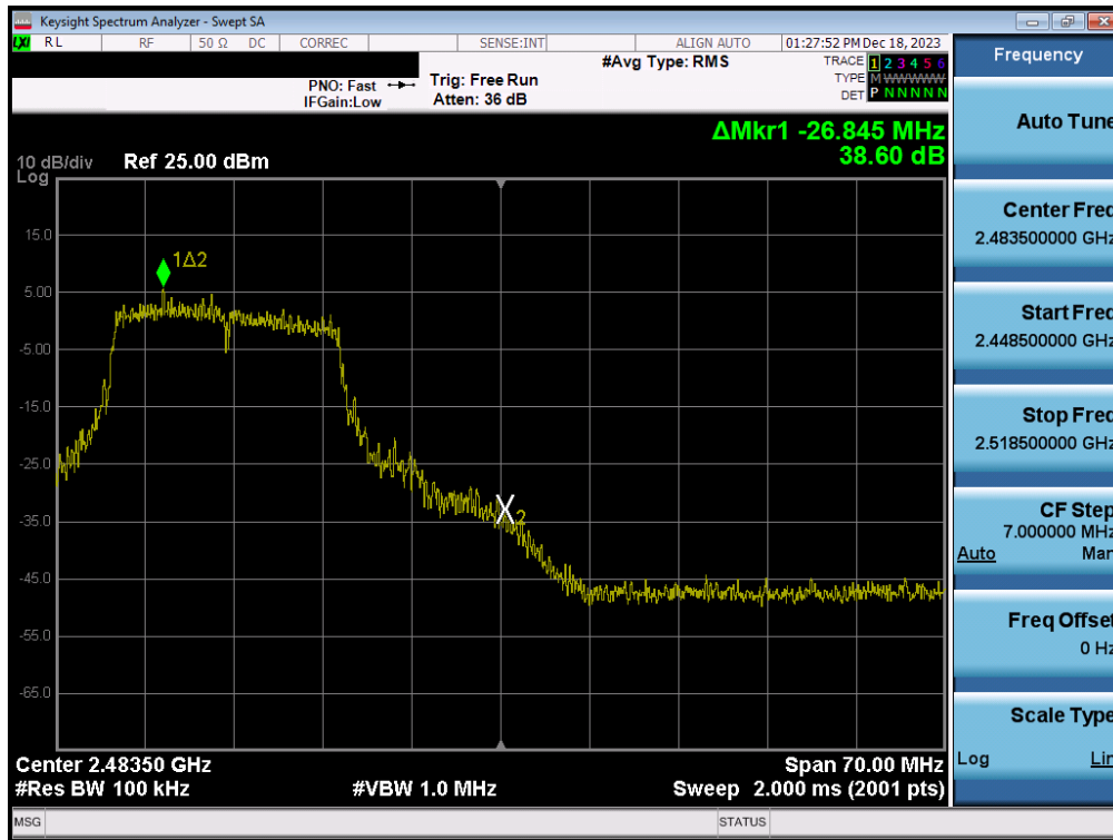
Plot 7-79. Band Edge Plot (802.11n (2.4GHz) – Ch. 11) – MIMO ANT2
