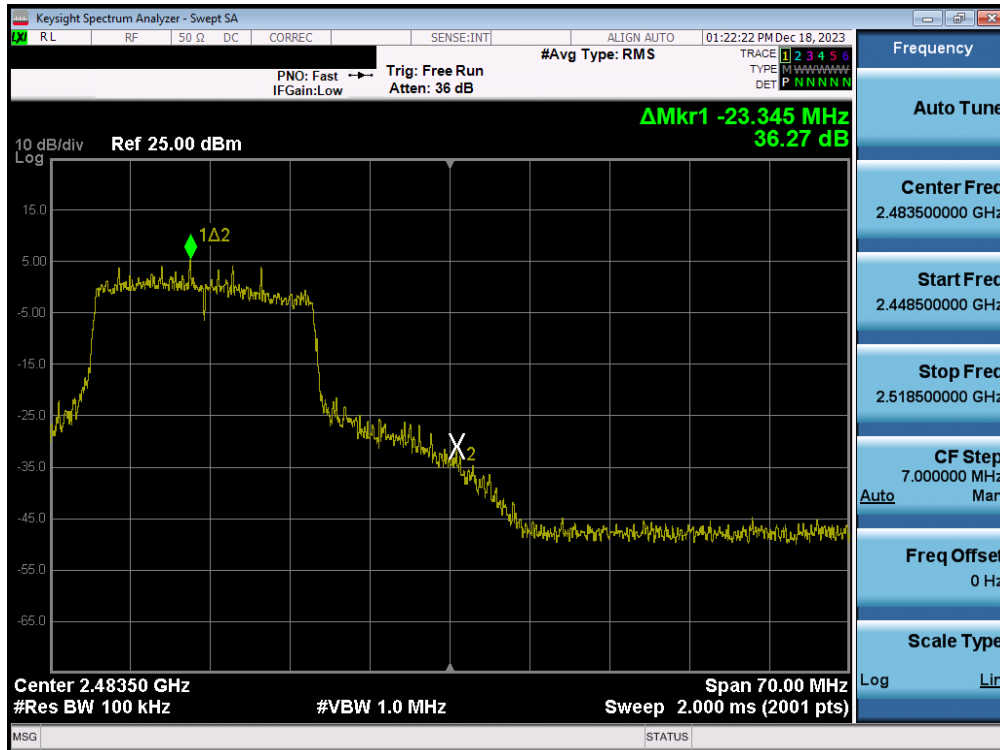
Plot 7-84. Band Edge Plot (802.11ax (2.4GHz) – Ch. 11) – MIMO ANT2
