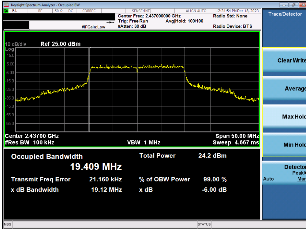
Plot 7-11. 6dB Bandwidth Plot (802.11ax (2.4GHz) – Ch. 6) – MIMO ANT1
