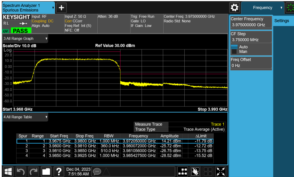
Plot 7-80. Upper ACP Plot (NR Band n77 - 10MHz CP-OFDM-QPSK – Full RB – Ant1)
