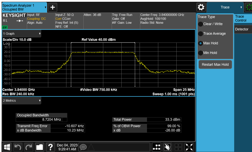
Plot 7-34. Occupied Bandwidth Plot (NR Band n77 - 10MHz \pi/2 BPSK - Full RB)
