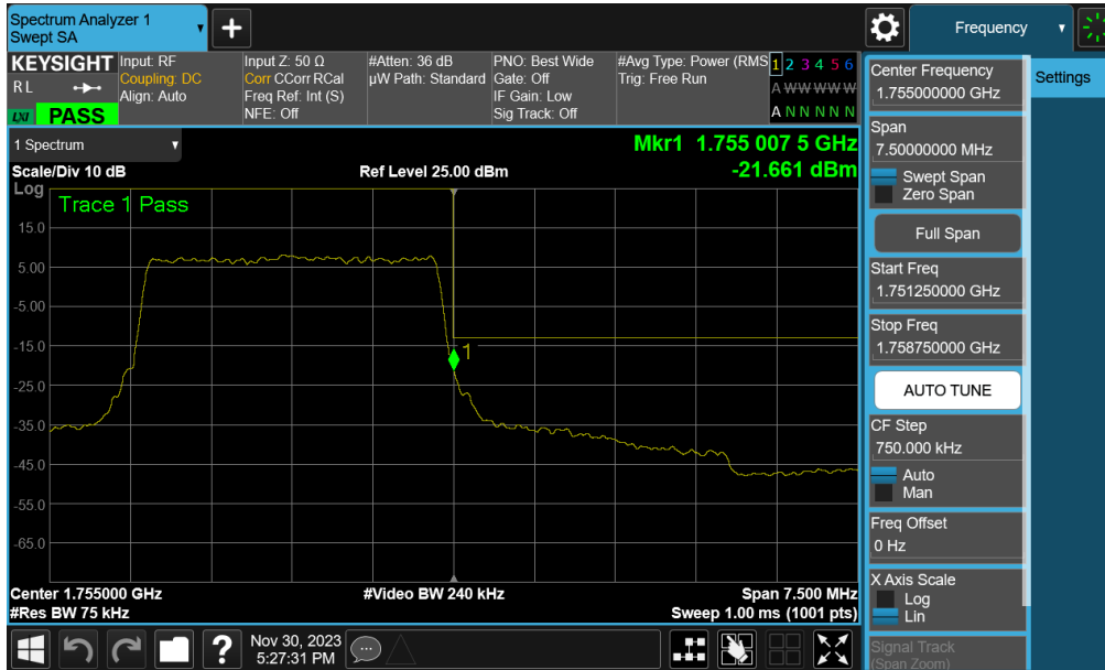
Plot 7-107. Upper Band Edge Plot (LTE Band 4 - 3MHz QPSK – Full RB - Ant B)
