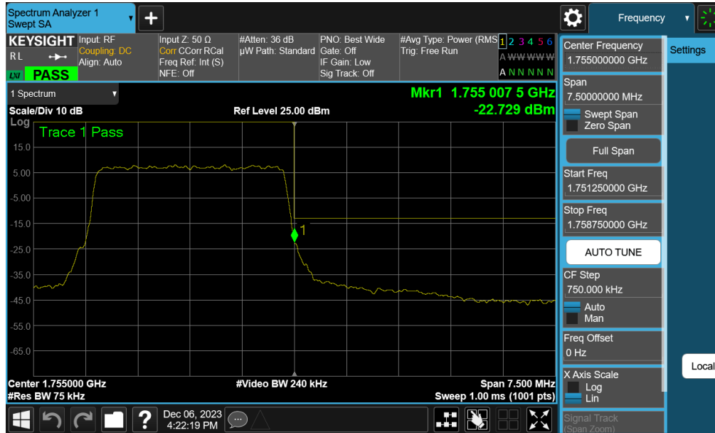
Plot 7-117. Upper Band Edge Plot (LTE Band 4 - 3MHz QPSK – Full RB - Ant F)
