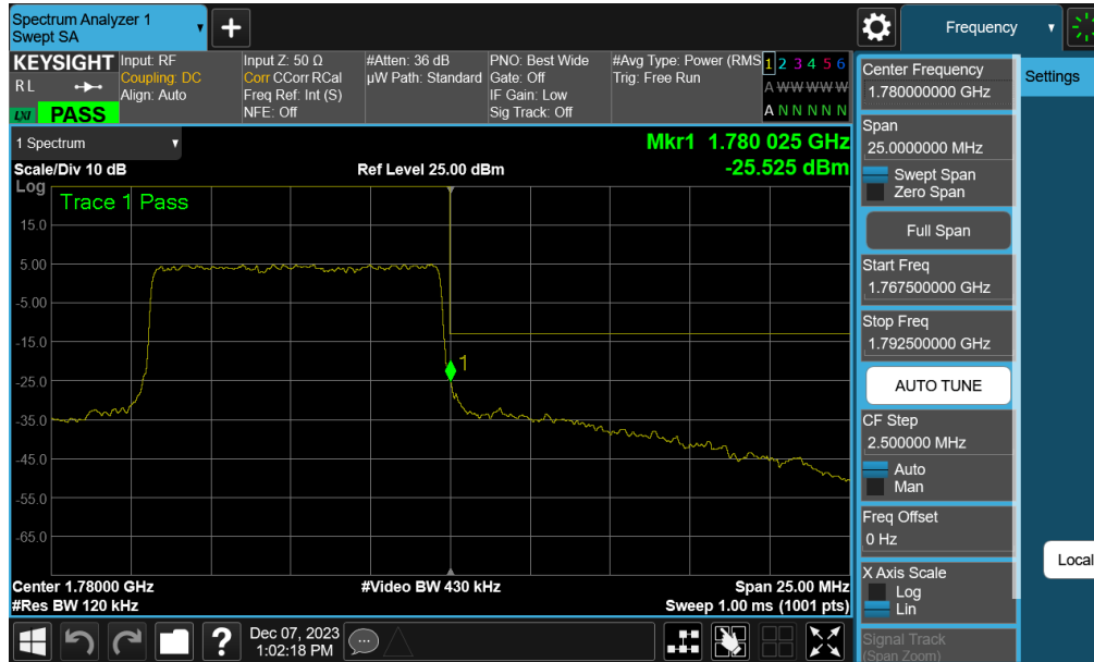
Plot 7-123. Upper Band Edge Plot (NR Band n66 – 10.0MHz - DFT-s BPSK - Full RB - Ant F)
