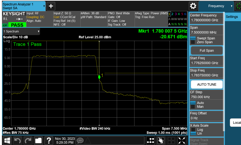
Plot 7-109. Upper Band Edge Plot (LTE Band 66 - 3MHz QPSK – Full RB - Ant B)
