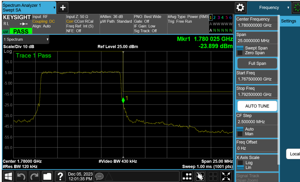
Plot 7-113. Upper Band Edge Plot (NR Band n66 – 10.0MHz - DFT-s BPSK - Full RB - Ant B)
