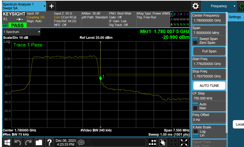
Plot 7-119. Upper Band Edge Plot (LTE Band 66 - 3MHz QPSK – Full RB - Ant F)
