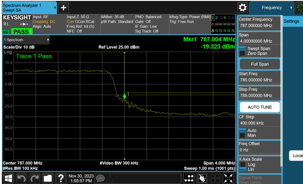
Plot 7-99. Upper Band Edge Plot (LTE Band 13 - 5MHz QPSK – Full RB - Ant A)
