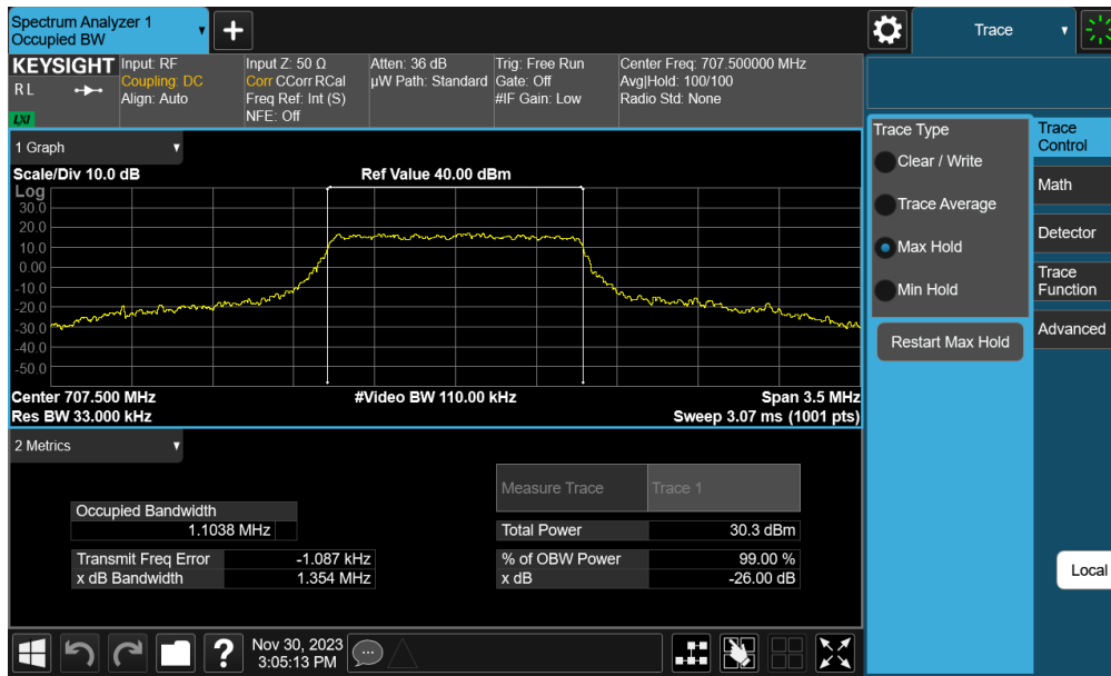
Plot 7-8. Occupied Bandwidth Plot (LTE Band 12 – 1.4MHz 16-QAM - Full RB – Ant A)
