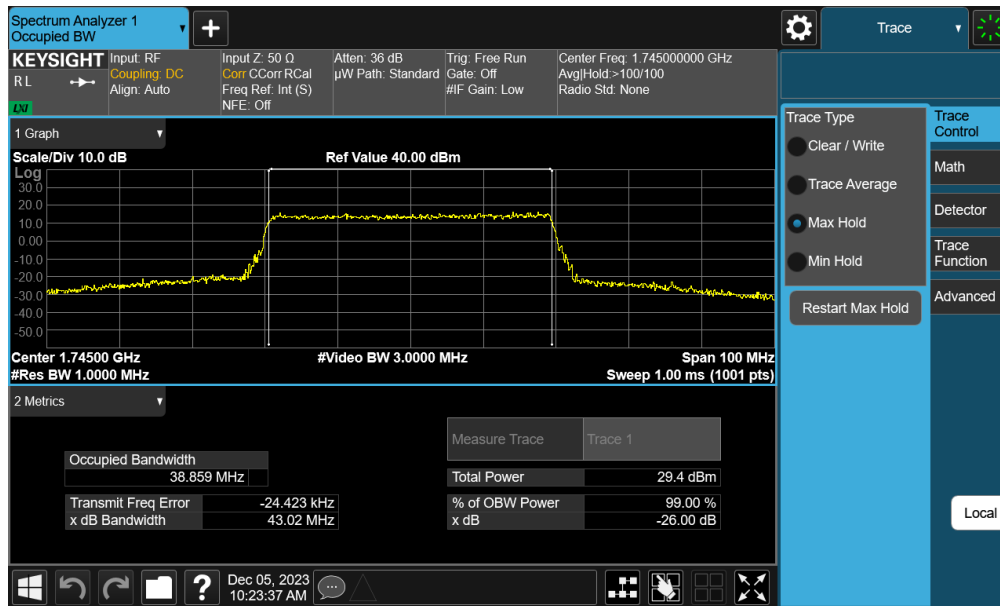
Plot 7-27. Occupied Bandwidth Plot (NR Band n66 - 40.0MHz CP-OFDM QPSK - Full RB – Ant B)
