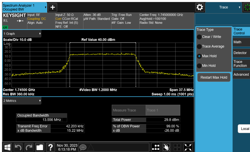
Plot 7-17. Occupied Bandwidth Plot (LTE Band 66/4 - 15MHz 16-QAM - Full RB - Ant B)
