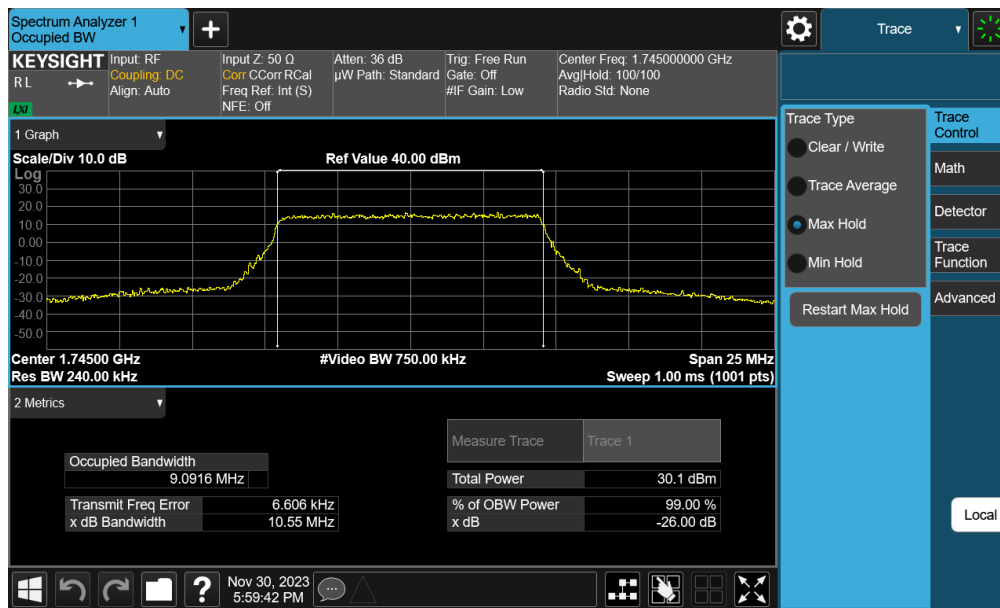
Plot 7-19. Occupied Bandwidth Plot (LTE Band 66/4 - 10MHz 16-QAM - Full RB - Ant B)
