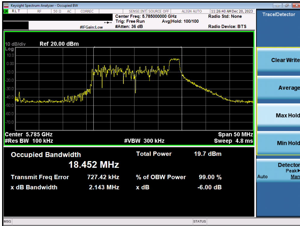
Plot 7-43. 6dB Bandwidth Plot MIMO ANT2 (20MHz BW 802.11ax – 26 Tones (UNII Band 3) – Ch. 157)
