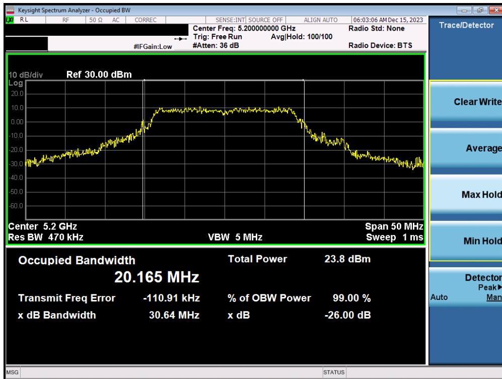
Plot 7-23. 26dB Bandwidth Plot MIMO ANT2 (20MHz BW 802.11n (UNII Band 1) – Ch. 40)
