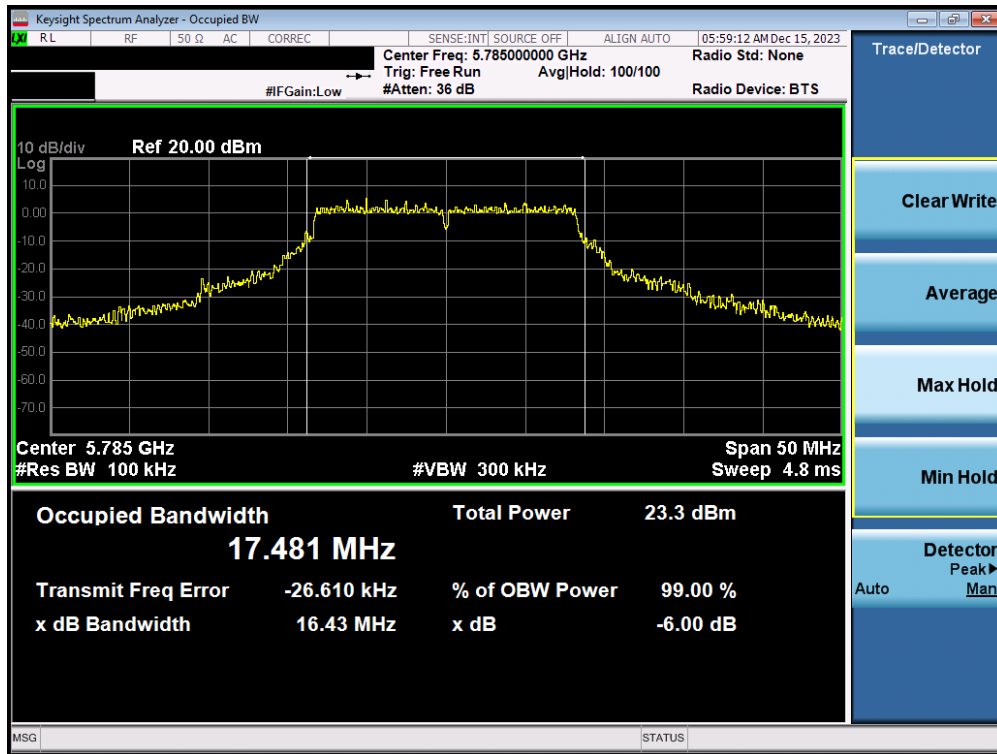
Plot 7-50. 6dB Bandwidth Plot MIMO ANT2 (802.11a (UNII Band 3) – Ch. 157)
