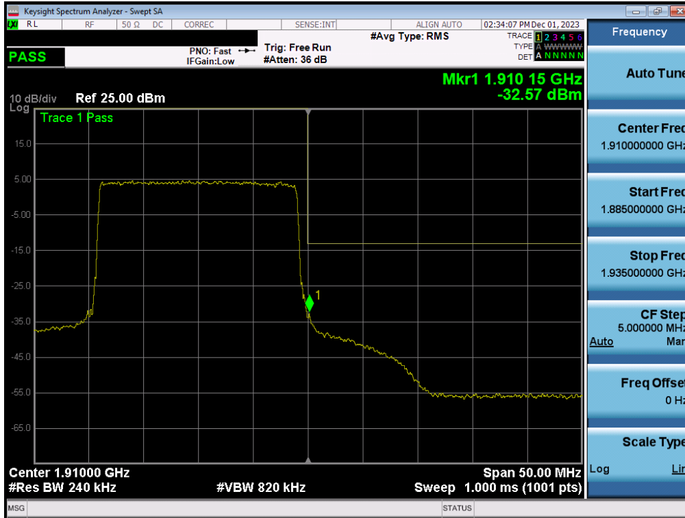
Plot 7-26. Upper Band Edge Plot (LTE Band 2 - 20MHz QPSK – Full RB - Ant1)
