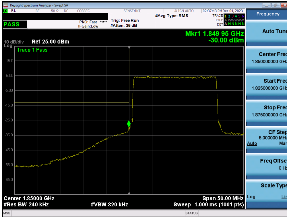
Plot 7-30. Lower Band Edge Plot (LTE Band 25/2 - 20MHz QPSK – Full RB - Ant2)
