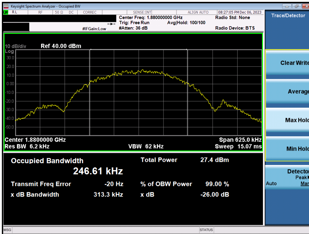
Plot 7-2. Occupied Bandwidth Plot (EDGE, Ch. 661 - Ant1)
