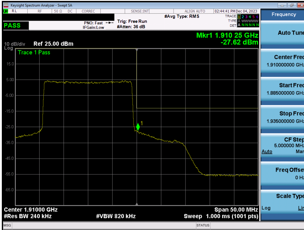
Plot 7-32. Upper Band Edge Plot (LTE Band 2 - 20MHz QPSK – Full RB - Ant2)
