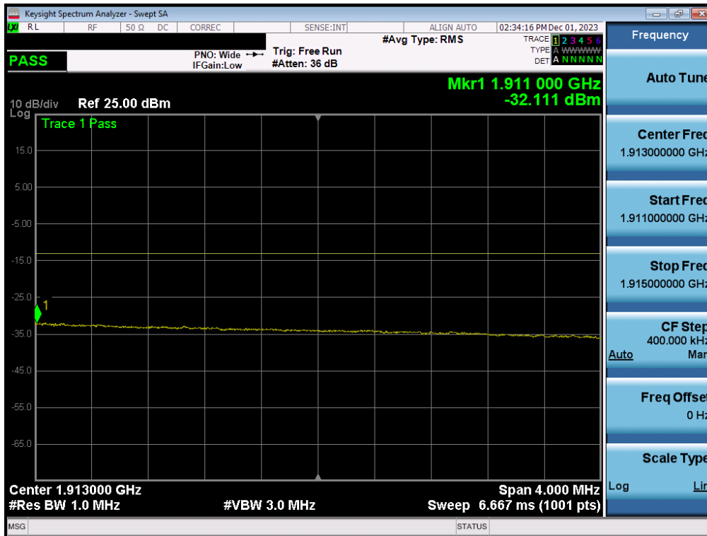
Plot 7-27. Extended Upper Band Edge Plot (LTE Band 2 - 20MHz QPSK – Full RB - Ant1)
