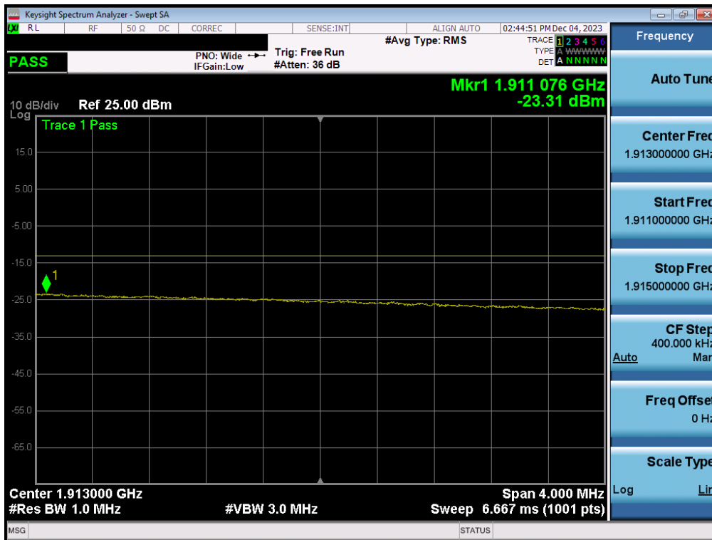
Plot 7-33. Extended Upper Band Edge Plot (LTE Band 2 - 20MHz QPSK – Full RB - Ant2)
