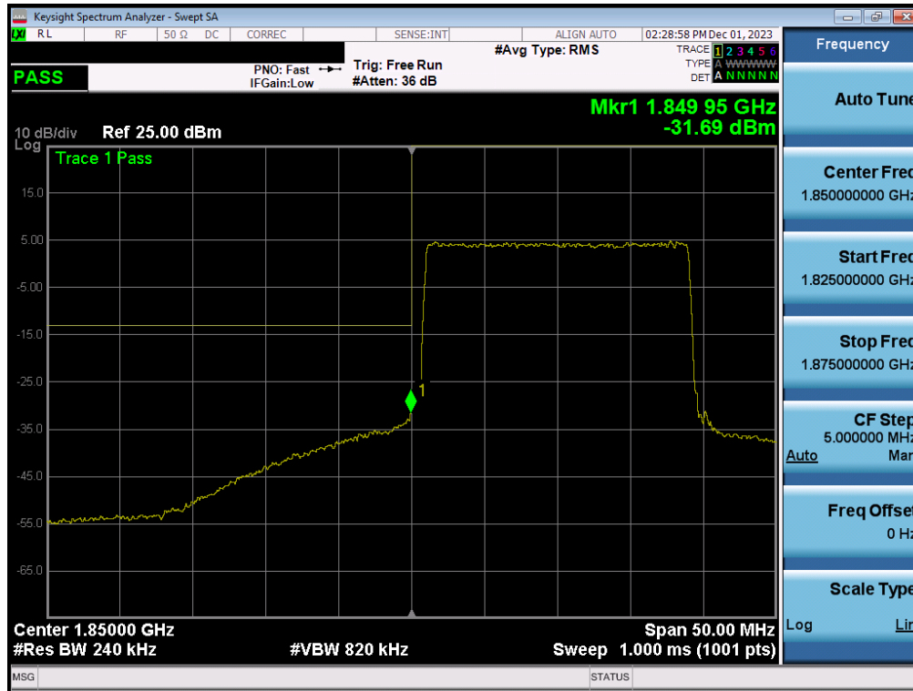
Plot 7-24. Lower Band Edge Plot (LTE Band 25/2 - 20MHz QPSK – Full RB - Ant1)
