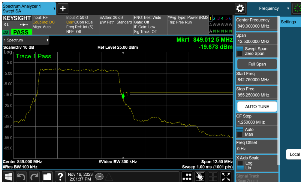
Plot 7-41. Upper Band Edge Plot (NR Band n5 – 5.0MHz BPSK - Full RB)
