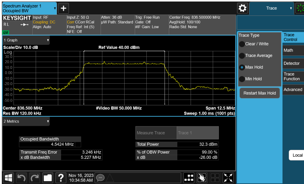
Plot 7-20. Occupied Bandwidth Plot (NR Band n5 - 5MHz \pi/2 BPSK - Full RB)
