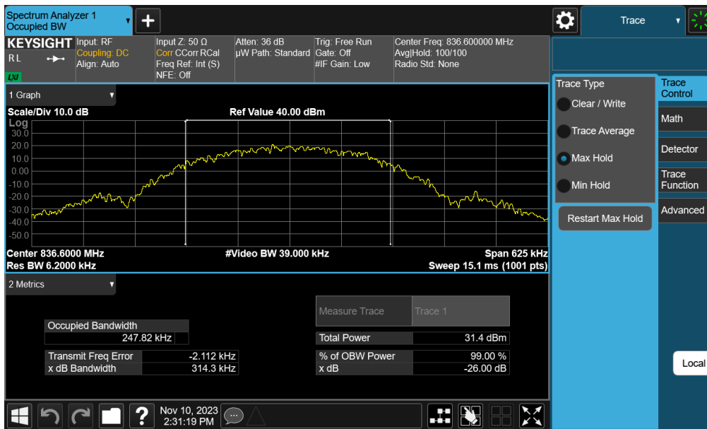
Plot 7-24. Occupied Bandwidth Plot (EDGE, Ch. 190)
