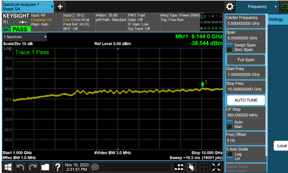
Plot 7-31. Conducted Spurious Plot (NR Band n5 - 20.0MHz - 1 RB - Mid Channel)
