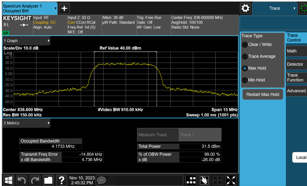
Plot 7-25. Occupied Bandwidth Plot (WCDMA, Ch. 4183)
