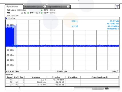
Channel move time = 0.757500 sClosing time =  $0.000625 \text{ s} \times 38 = 0.023750 \text{ s}$
