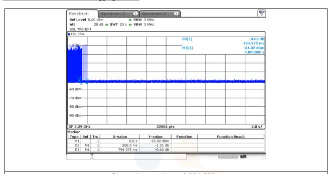
Channel move time =  $0.794 \frac{375 \text{ s}}{625 \text{ s}}$ Closing time =  $0.000 625 \text{ s} \times 65 = 0.040 625 \text{ s}$
