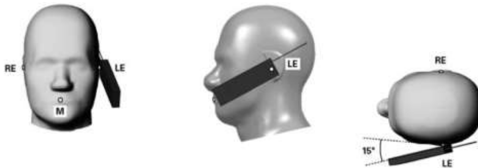
Figure 8.5. Tilt 15° position of the wireless device
