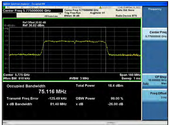
802.11ac_VHT80 UNII 3 BAND 26 dB Bandwidth (CH 155)
