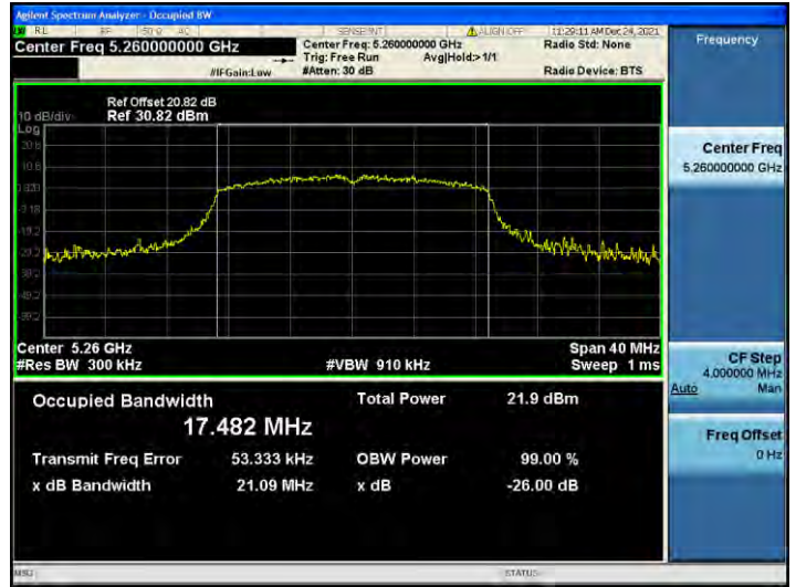
802.11n_HT20 UNII 3 BAND 26 dB Bandwidth (CH 165)
