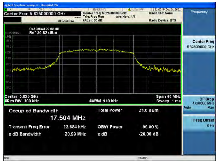
802.11n_HT20 UNII 3 BAND 26 dB Bandwidth (CH 165)
