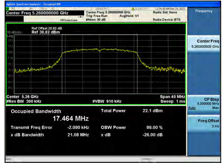
802.11ac_VHT20 UNII 3 BAND 26 dB Bandwidth(CH 149)
