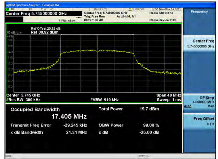
802.11ac_VHT20 UNII 3 BAND 26 dB Bandwidth(CH 149)
