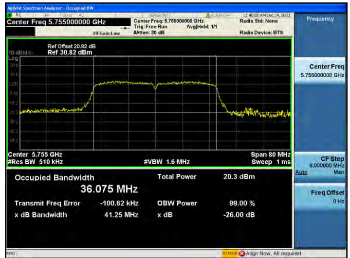
802.11n_HT40 UNII 3 BAND 26 dB Bandwidth (CH 151)
