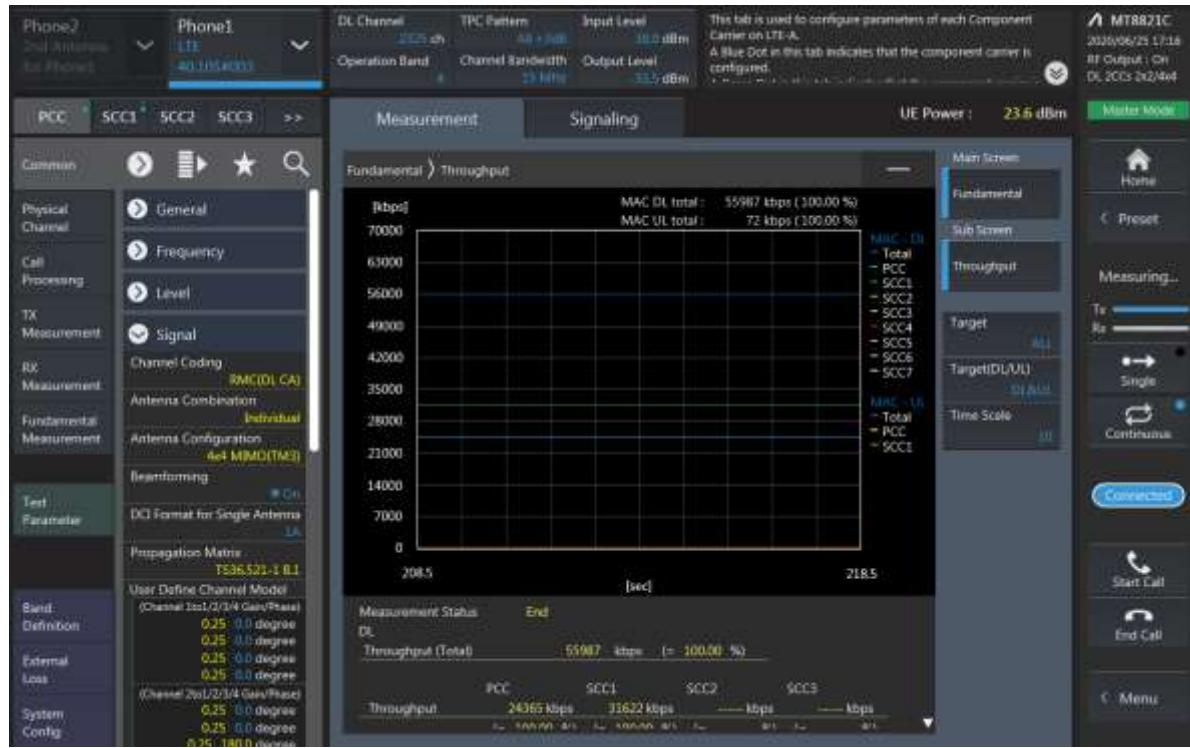
SCC Setting : Channel/ RB/ BW/ Modulation and call Connection
