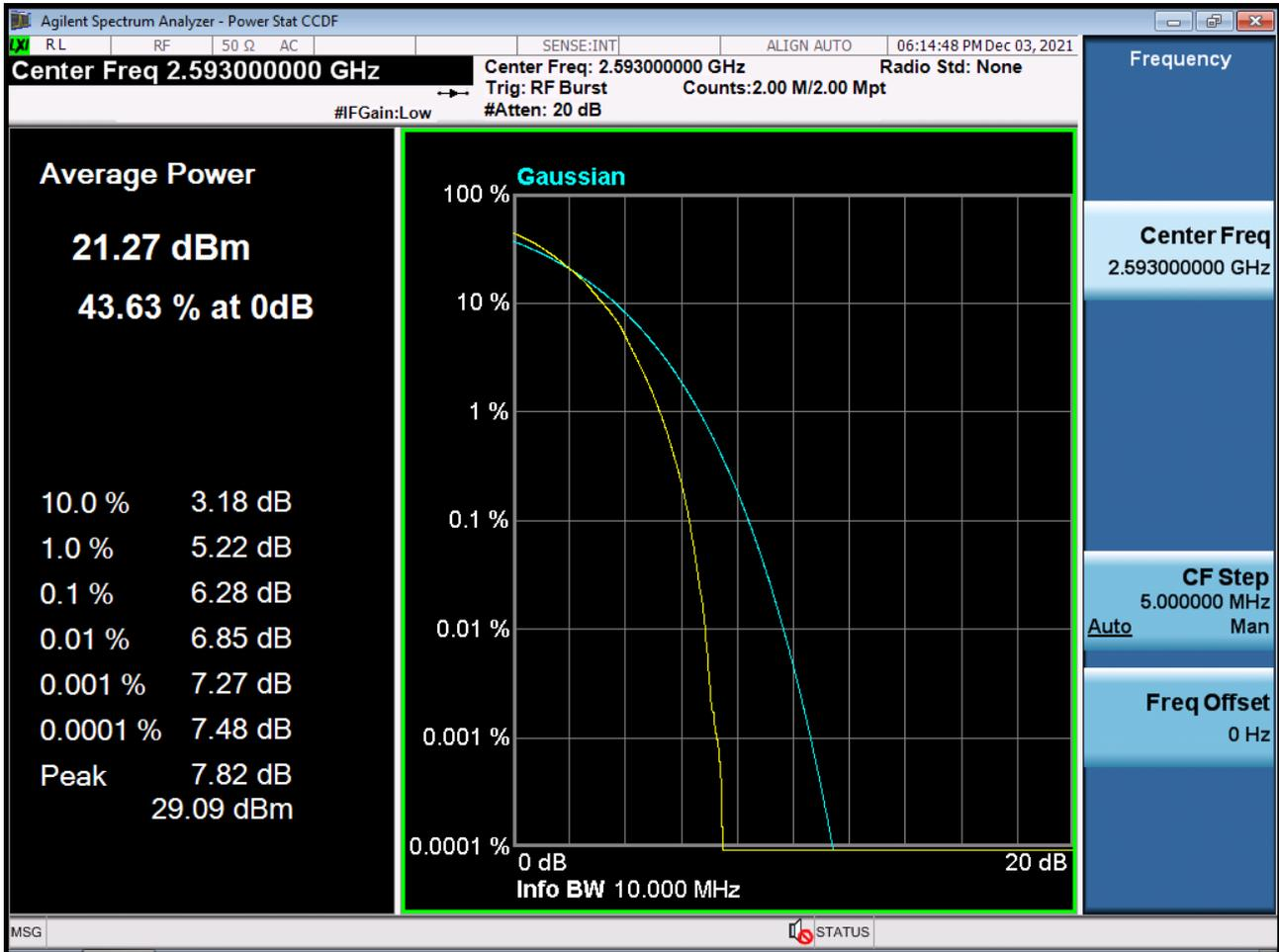
PAR Plot (10 M BW\_Ch.40620\_256QAM\_RB50\_0) (POWER CLASS 3)
