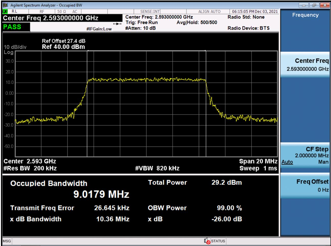
Occupied Bandwidth Plot (10 MHz Ch.40620 256-QAM RB 50) (POWER CLASS 3)
