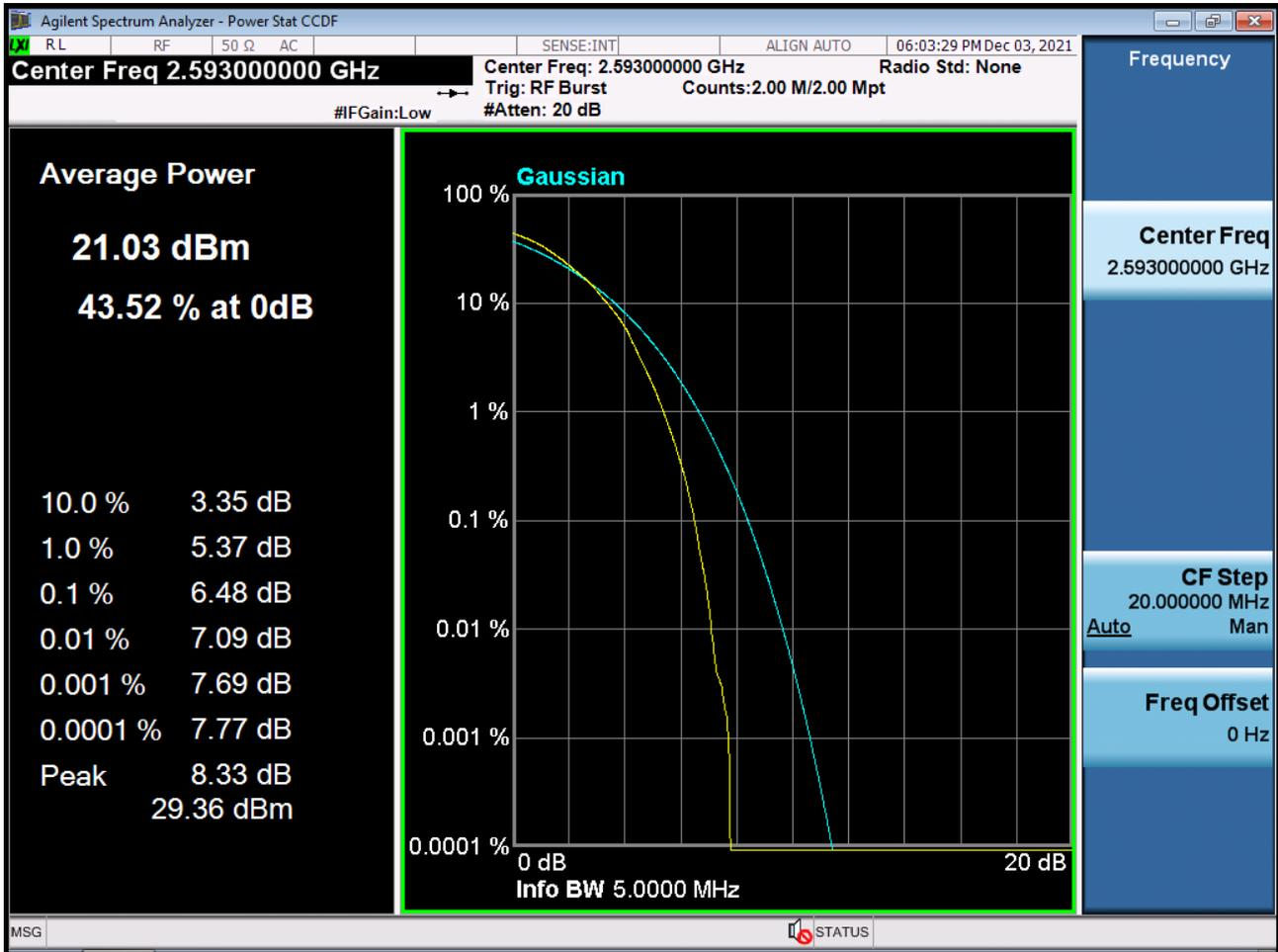
PAR Plot (5 M BW\_Ch.40620\_256QAM\_RB25\_0) (POWER CLASS 3)
