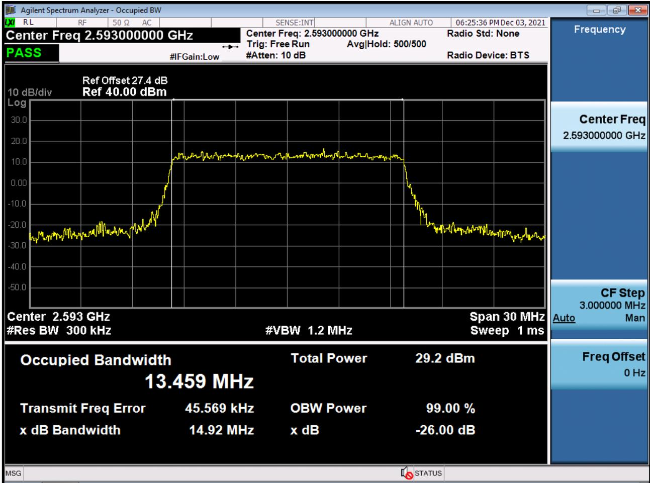
Occupied Bandwidth Plot (15 MHz Ch.40620 256-QAM RB 75) (POWER CLASS 3)
