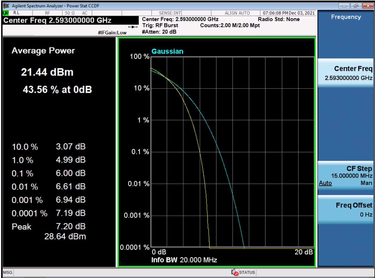
PAR Plot (20 M BW\_Ch.40620\_256QAM\_RB100\_0) (POWER CLASS 3)
