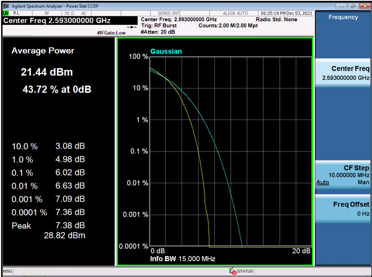
PAR Plot (15 M BW\_Ch.40620\_256QAM\_RB75\_0) (POWER CLASS 3)
