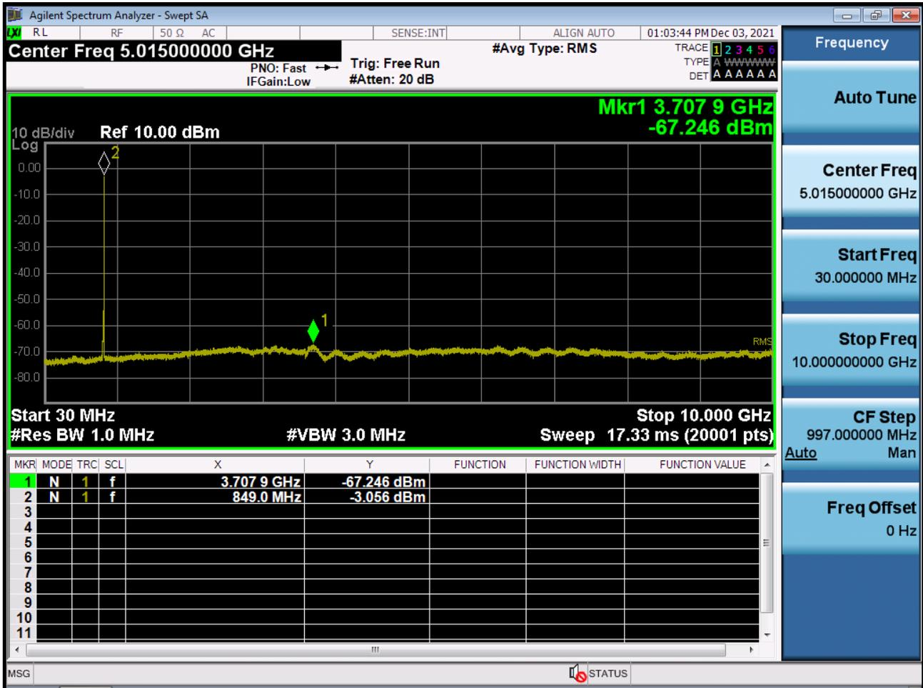
BAND 26. Conducted Spurious (26865ch\_15 MHz\_QPSK\_RB 1\_0)
