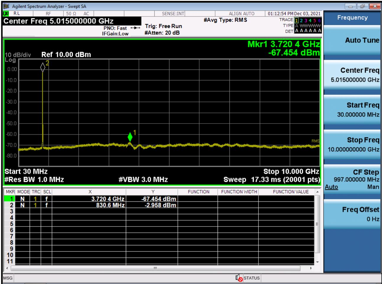
BAND 26. Conducted Spurious (26965ch\_15 MHz\_QPSK\_RB 1\_0)
