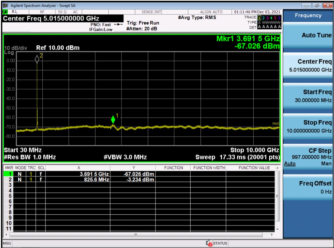
BAND 26. Conducted Spurious (26915ch\_15 MHz\_QPSK\_RB 1\_0)
