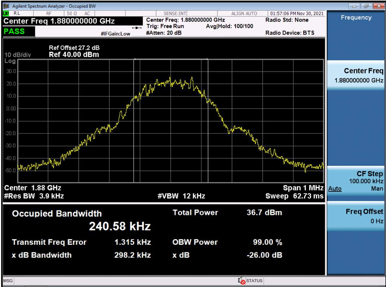
■ GSM1900 MODE (810 CH.) Occupied Bandwidth
