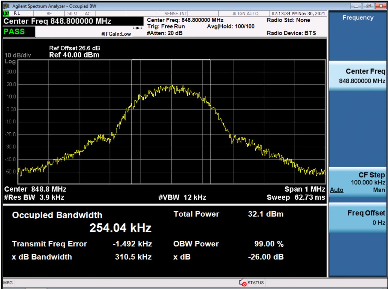
■ GSM1900 MODE (512 CH.) Occupied Bandwidth
