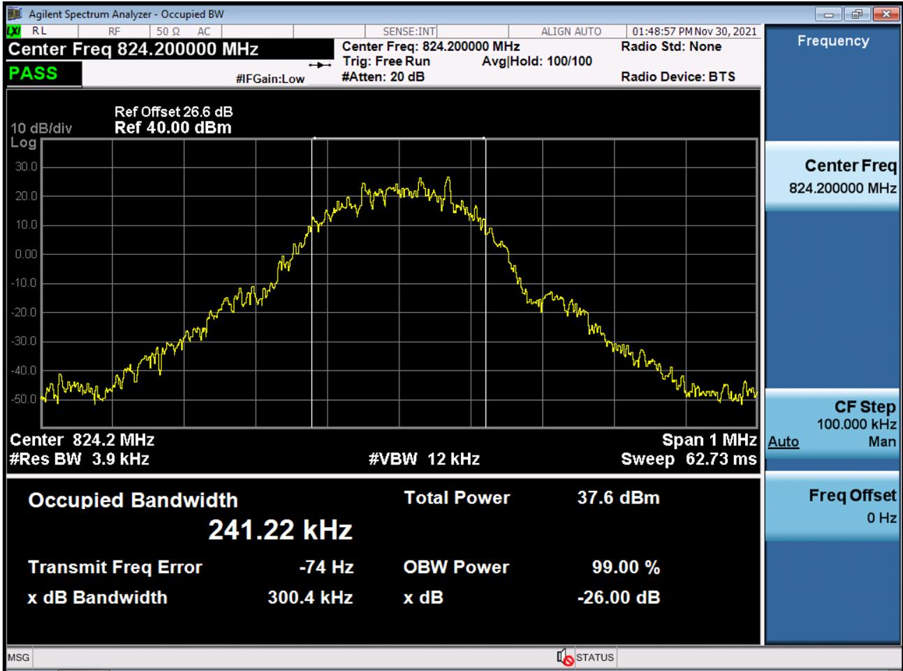
■ GSM850 MODE (190 CH.) Occupied Bandwidth
