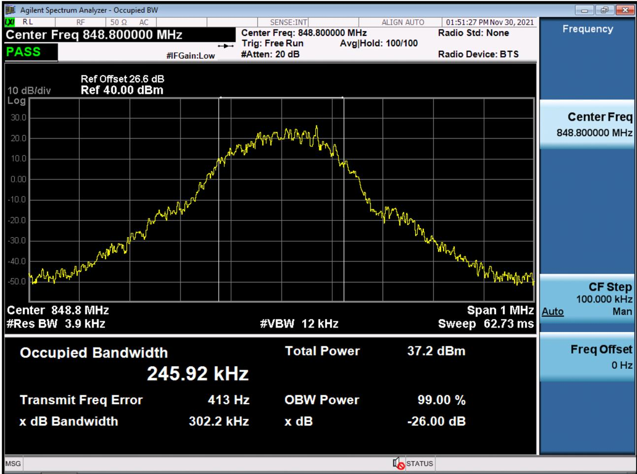
■ GSM850 EDGE (251 CH.) Occupied Bandwidth
