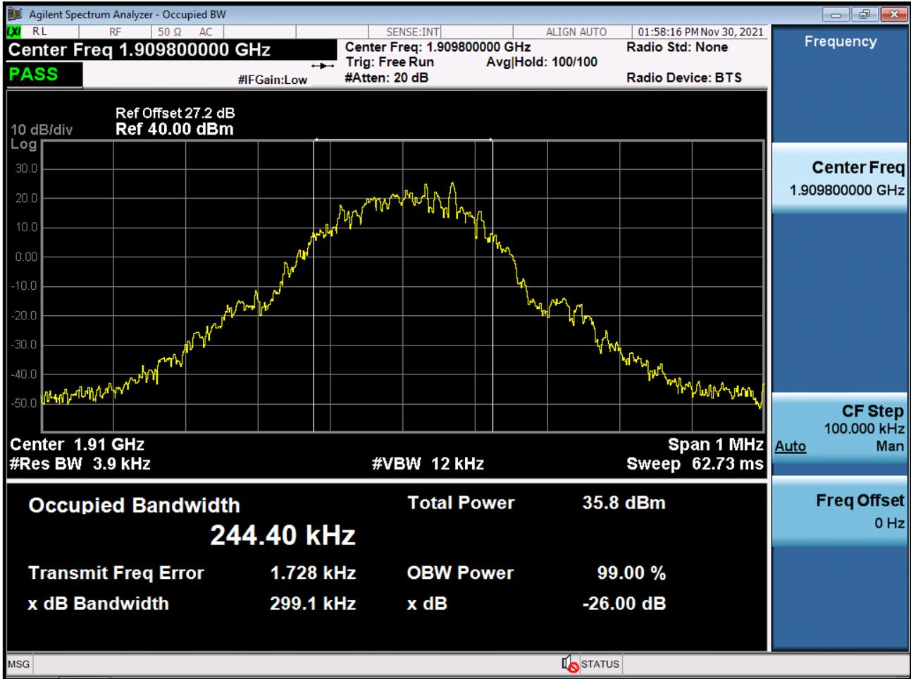
■ GSM1900 EDGE (810 CH.) Occupied Bandwidth
