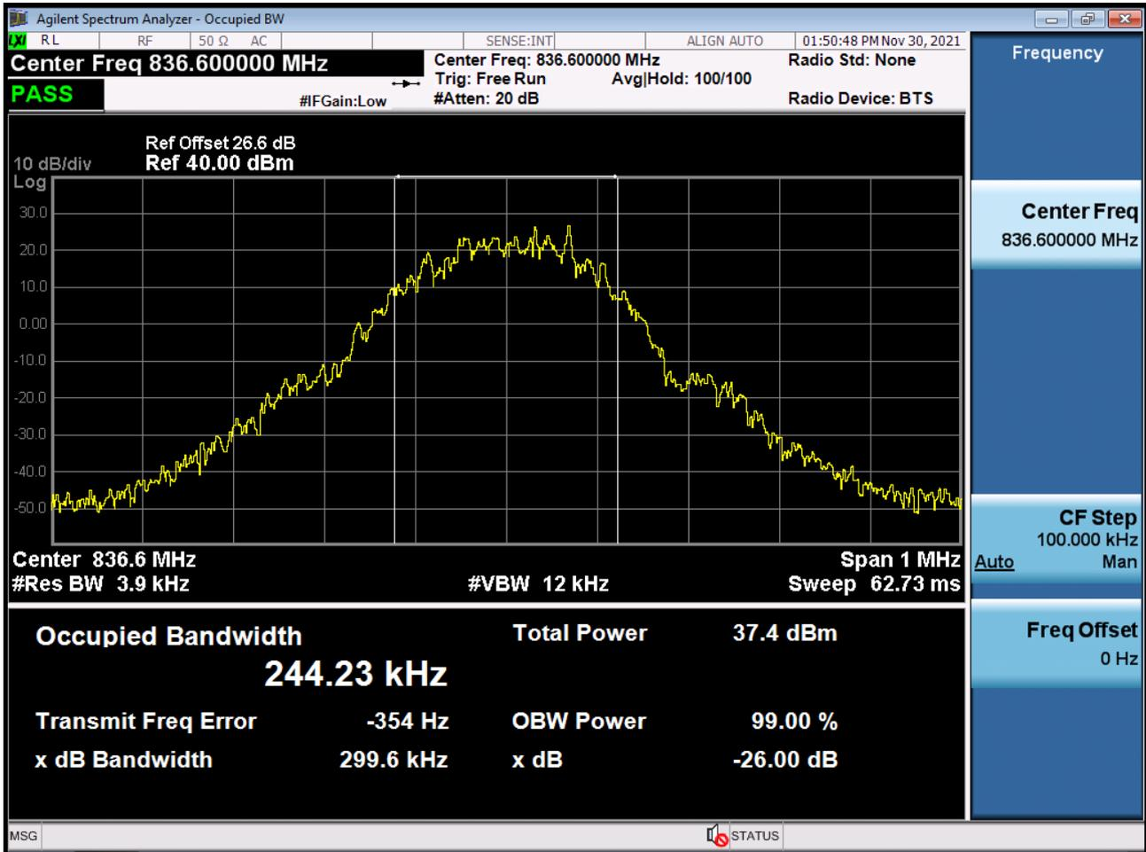
■ GSM850 MODE (251 CH.) Occupied Bandwidth
