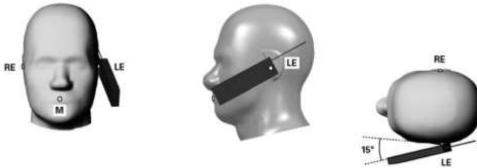
Figure 8.5. Tilt 15° position of the wireless device
