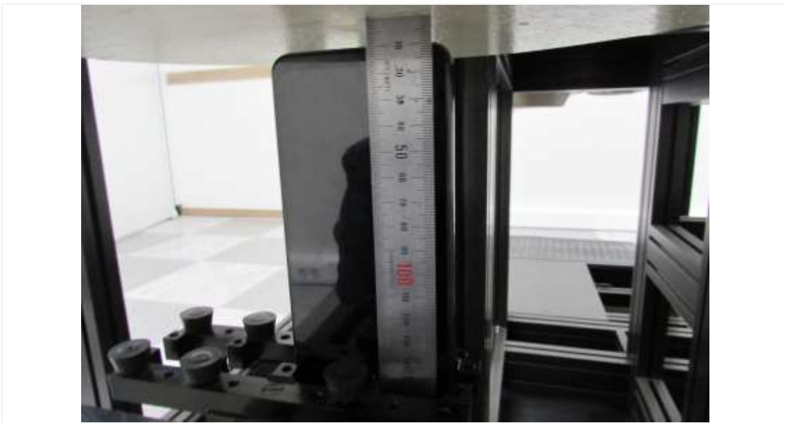
Distance of 10 mm from the EUT
