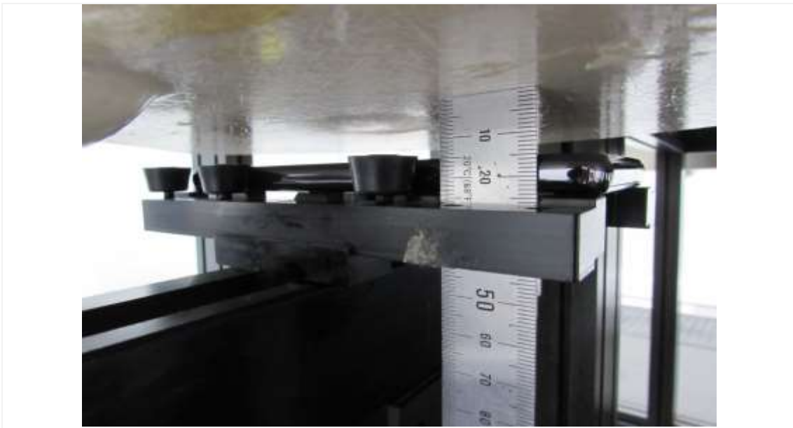
Distance of 15 mm from the EUT
