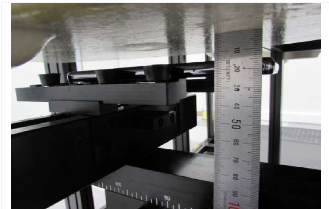
Distance of 15 mm from the EUT
