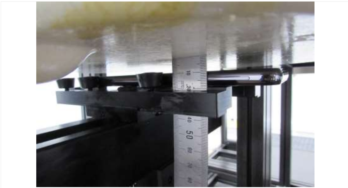
Distance of 10 mm from the EUT for Main Ant#1
