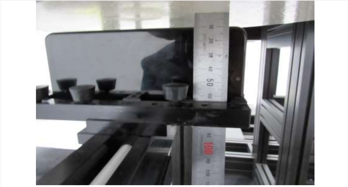
Distance of 10 mm from the EUT
