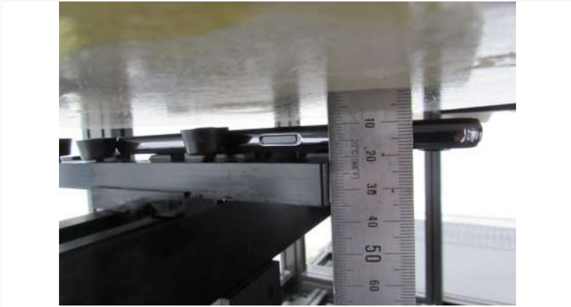
Distance of 10 mm from the EUT
