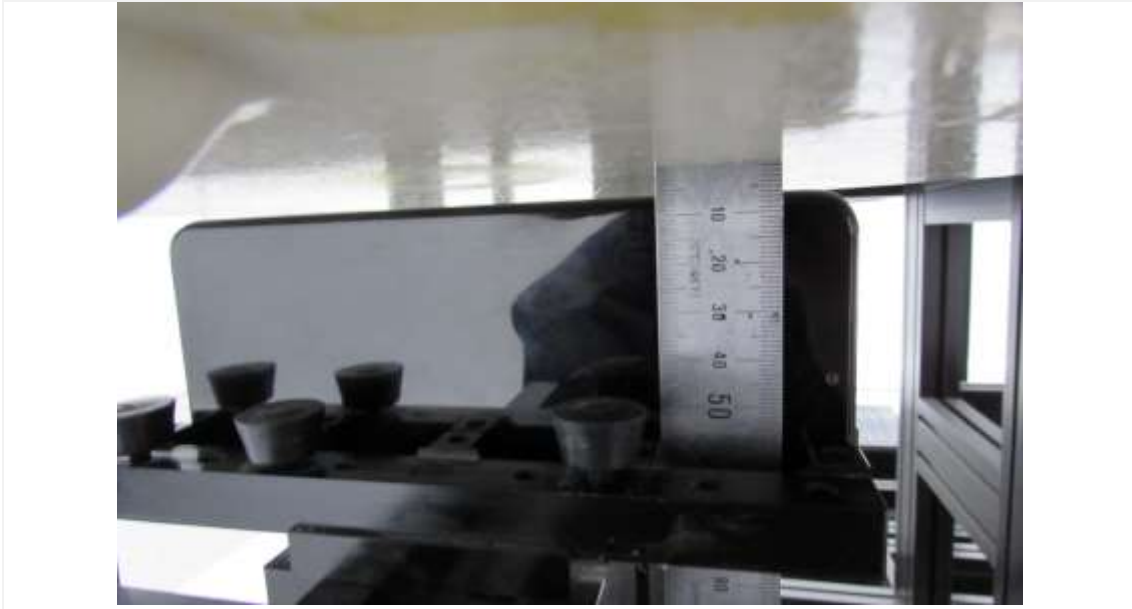
Distance of 6 mm from the EUT for Main Ant#2
