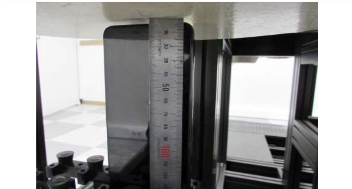
Distance of 3 mm from the EUT for Main Ant#1
