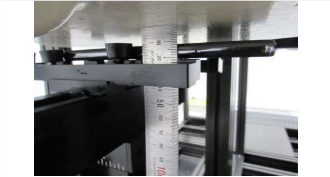
Distance of 12 mm from the EUT for Main Ant#2
