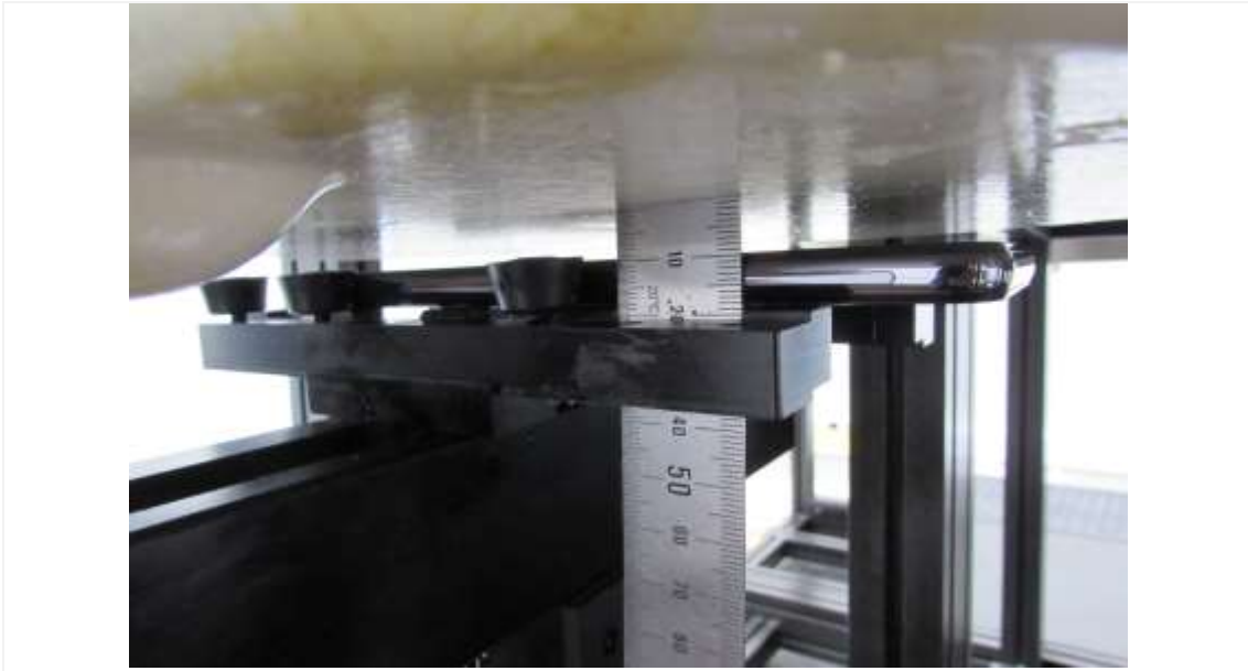
Distance of 10 mm from the EUT
