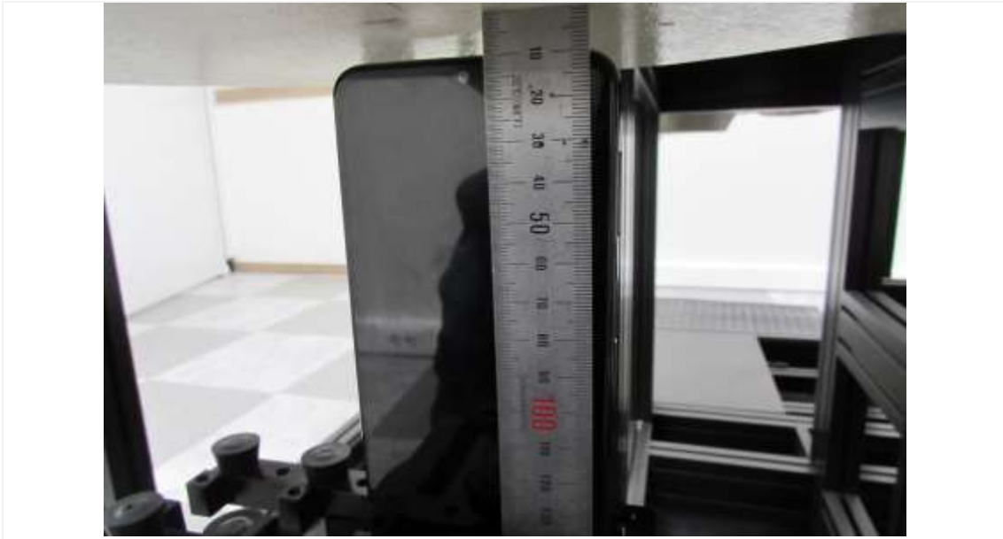
Distance of 10 mm from the EUT
