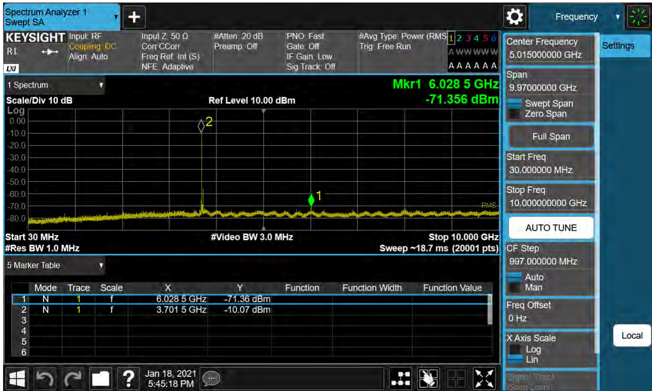
Sub6 n77. Conducted Spurious Plot_1 (649334ch_80MHz_BPSK)
