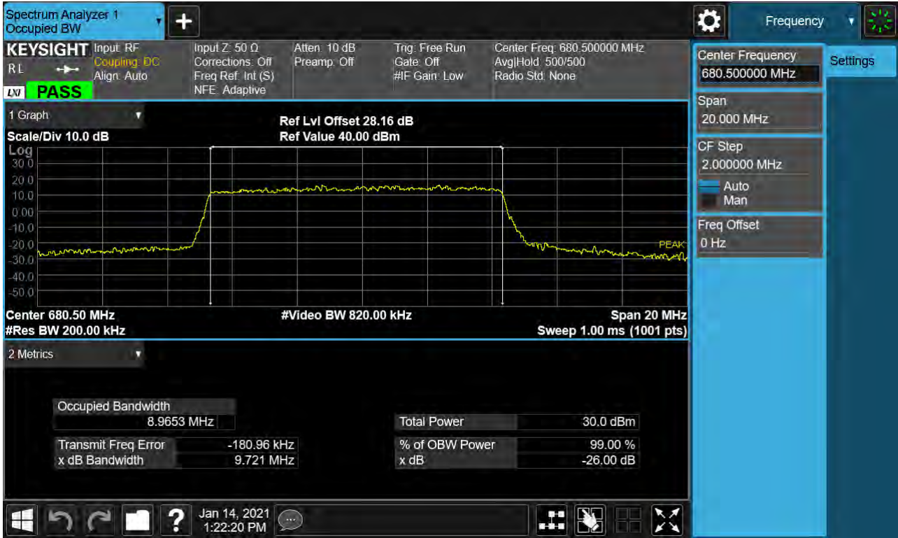
Sub6 n71. Occupied Bandwidth Plot (10M BW Ch.136100 16QAM_ RB52_0)
