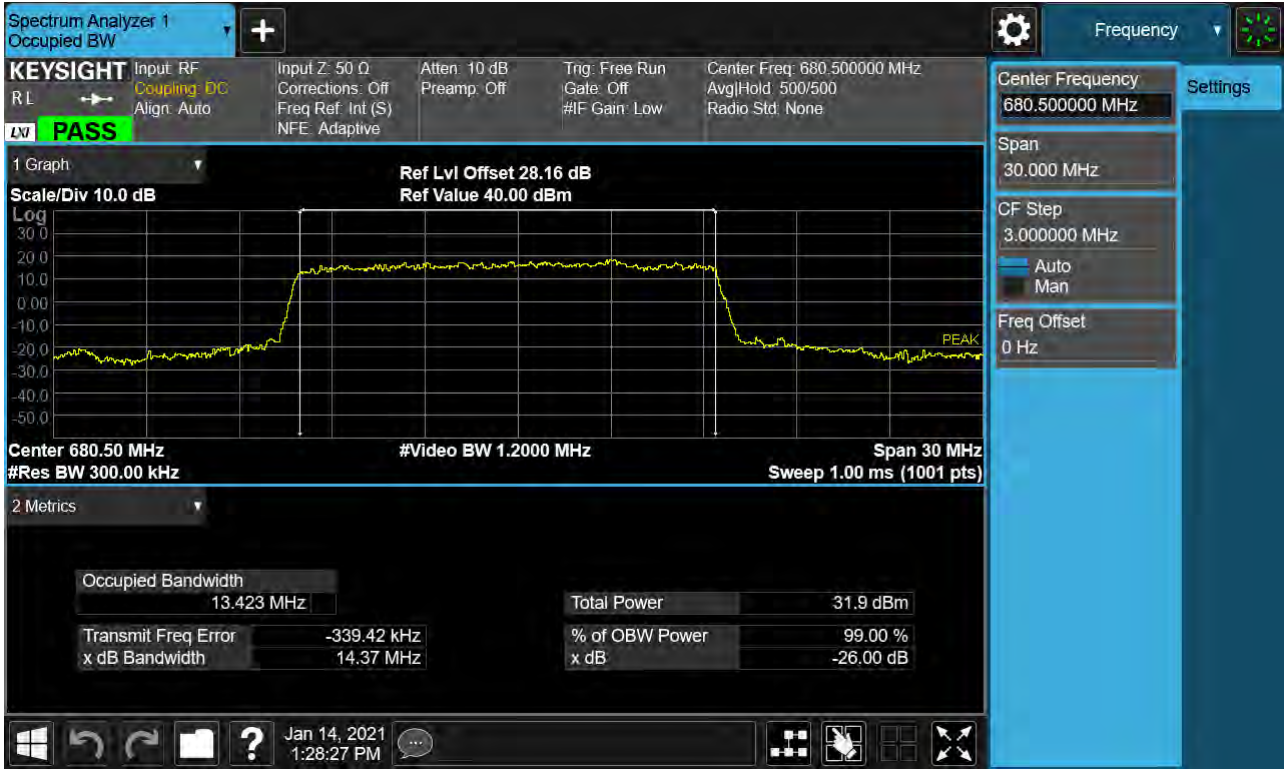
Sub6 n71. Occupied Bandwidth Plot (15M BW Ch.136100 BPSK_ RB79_0)
