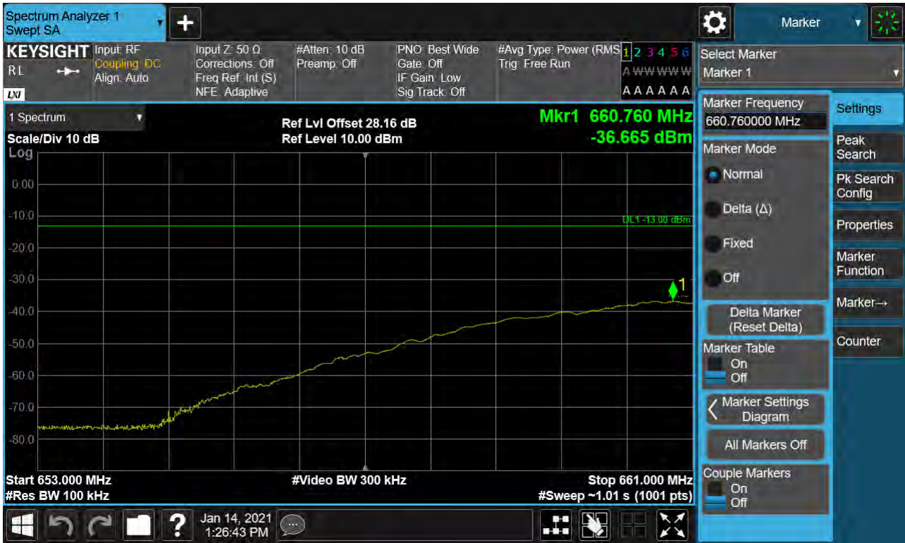
Sub6 n71. Lower Extended Band Edge Plot (15M BW Ch.134100 BPSK_RB79_0)
