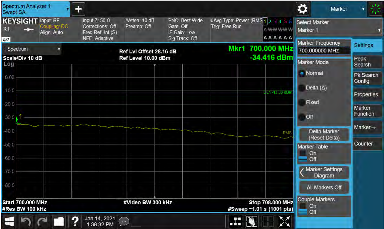
Sub6 n71. Upper Extended Band Edge Plot (20M BW Ch.137600 BPSK_RB106_0)
