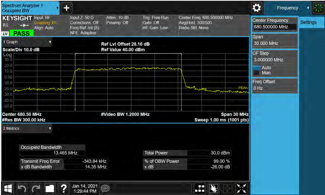
Sub6 n71. Occupied Bandwidth Plot (15M BW Ch.136100 64QAM_ RB79_0)
