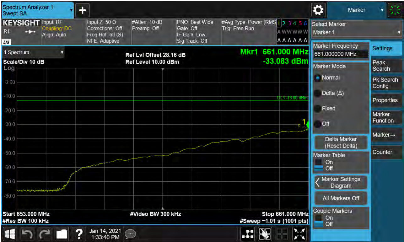
Sub6 n71. Lower Extended Band Edge Plot (20M BW Ch.134600 BPSK_RB106_0)
