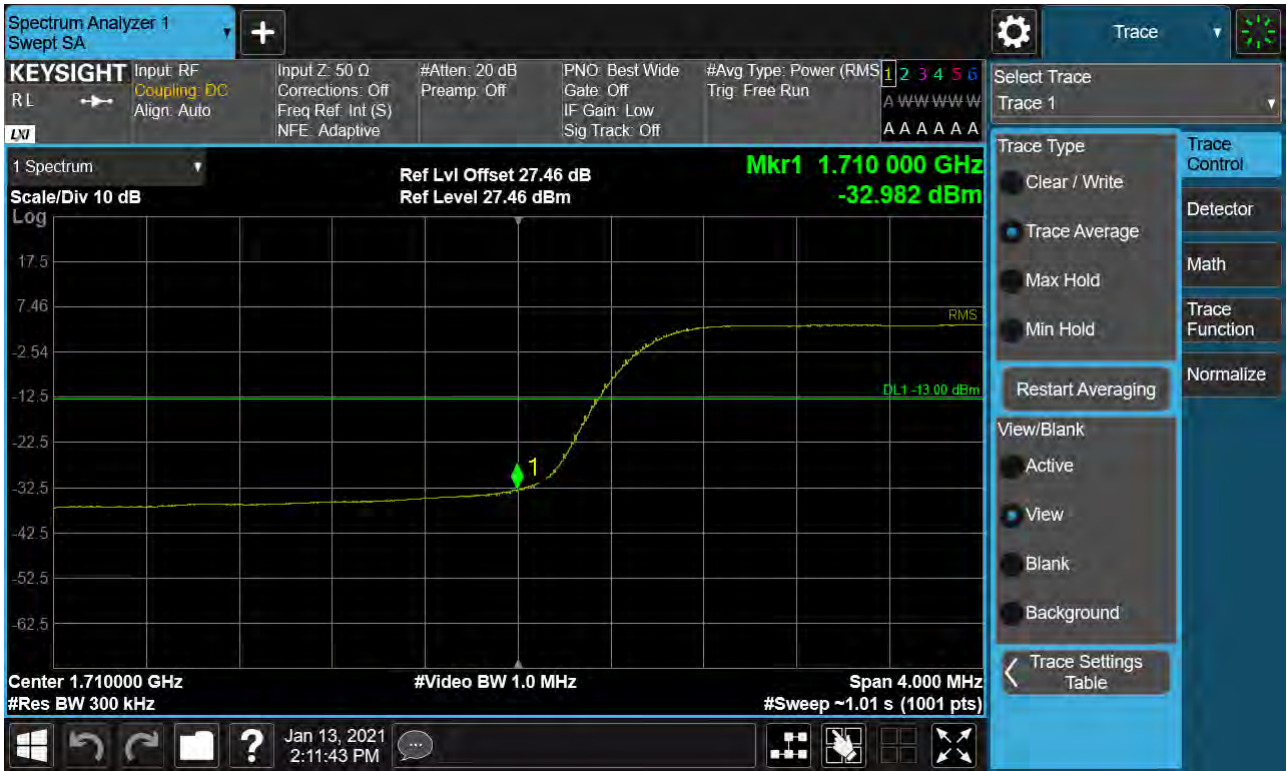
Sub6 n66. Lower Band Edge Plot (30M BW Ch.345000 BPSK RB 160_0) -2
