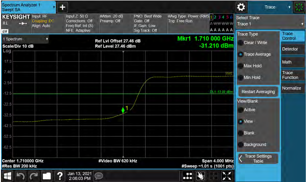
Sub6 n66. Lower Band Edge Plot (20M BW Ch.344000 BPSK RB 106_0) -2
