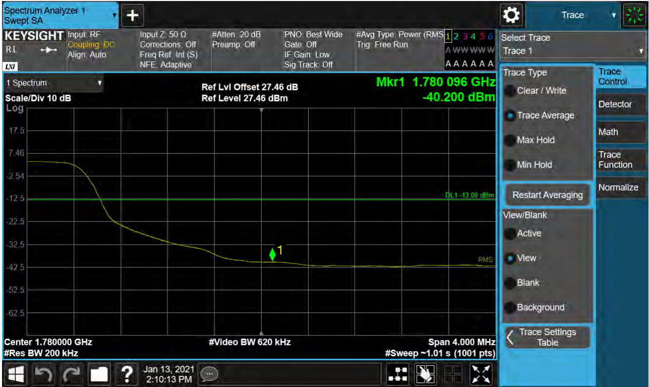
Sub6 n66. Upper Band Edge Plot (20M BW Ch.354000 BPSK_RB106_0) -2
