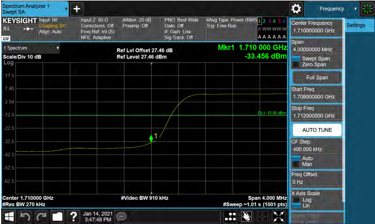
Sub6 n66. Lower Band Edge Plot (25M BW Ch.344500 BPSK RB 133_0) -2
