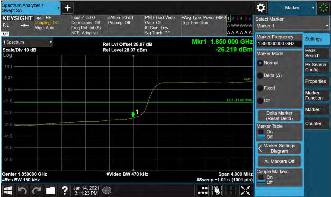
Sub6 n25. Lower Band Edge Plot (15M BW Ch.371500 BPSK_RB79_Offset 0) -1
