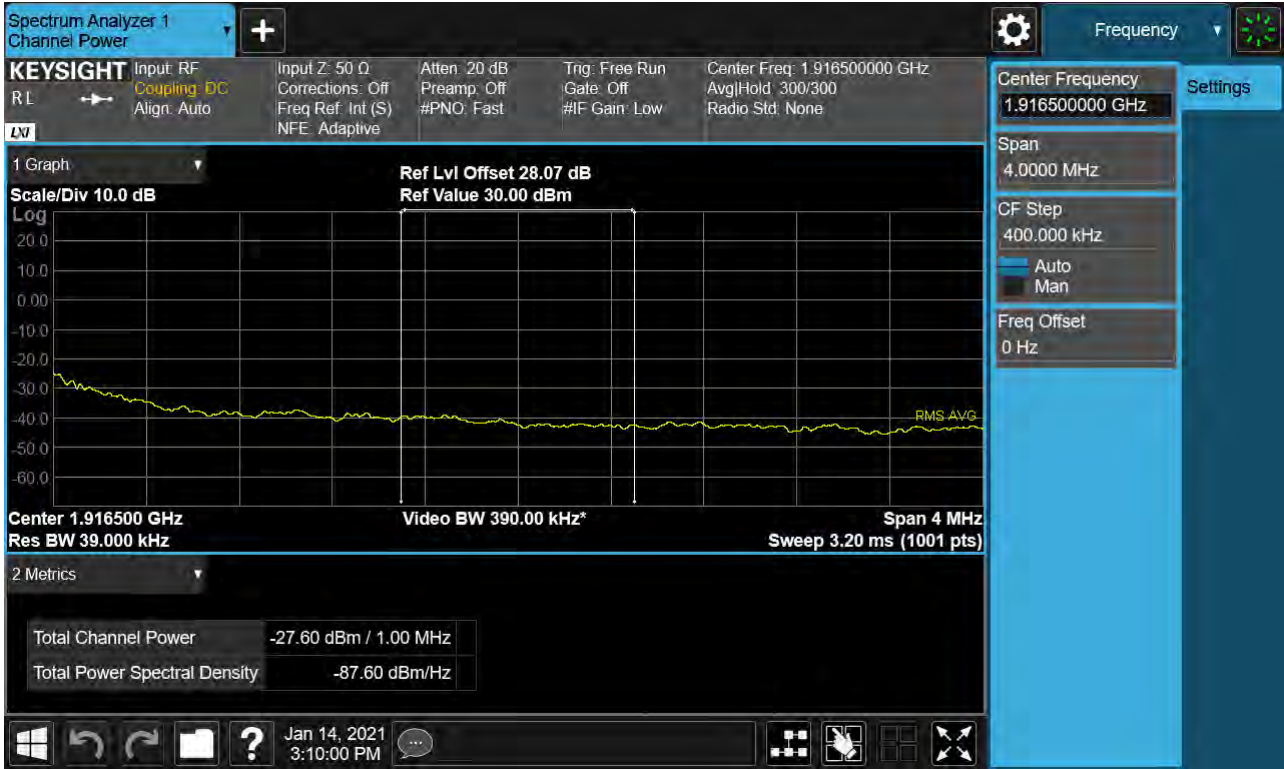
Sub6 n25. Upper Extended Band Edge Plot (10M BW Ch.382000 BPSK_RB52_0) -2
