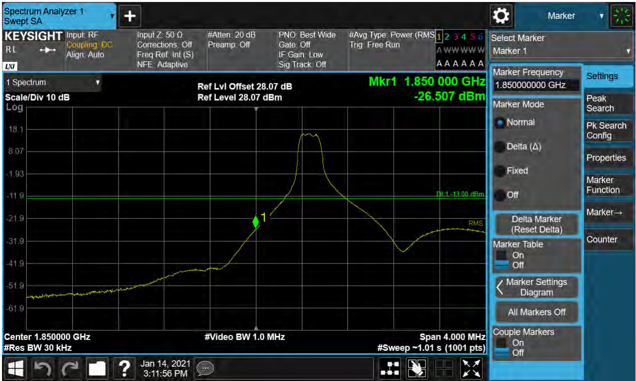
Sub6 n25. Lower Band Edge Plot (15M BW Ch.371500 BPSK_RB1_Offset 0)
