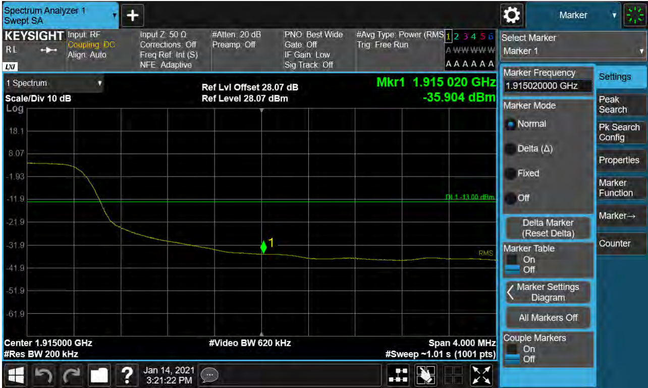
Sub6 n25. Upper Band Edge Plot (20M BW Ch.381000 BPSK_RB106_Offset 0) -1
