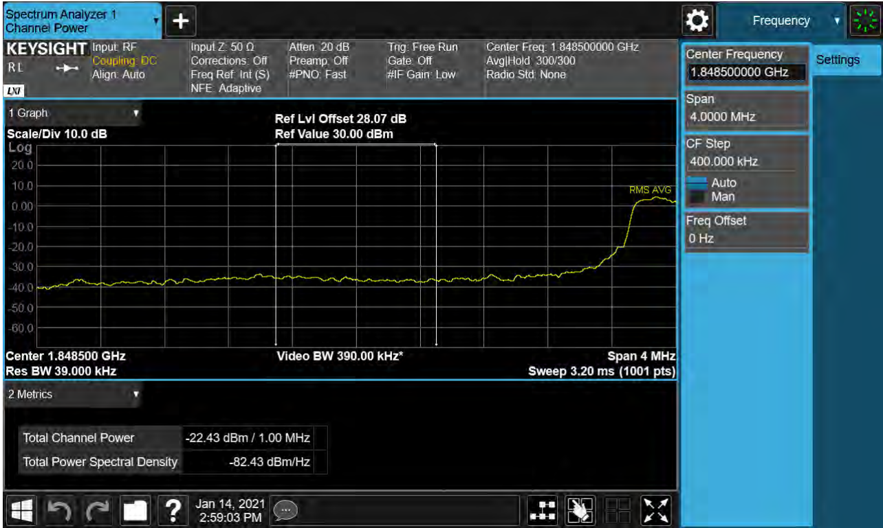
Sub6 n25. Lower Extended Band Edge Plot (5M BW Ch.370500 BPSK_RB25_0) -2
