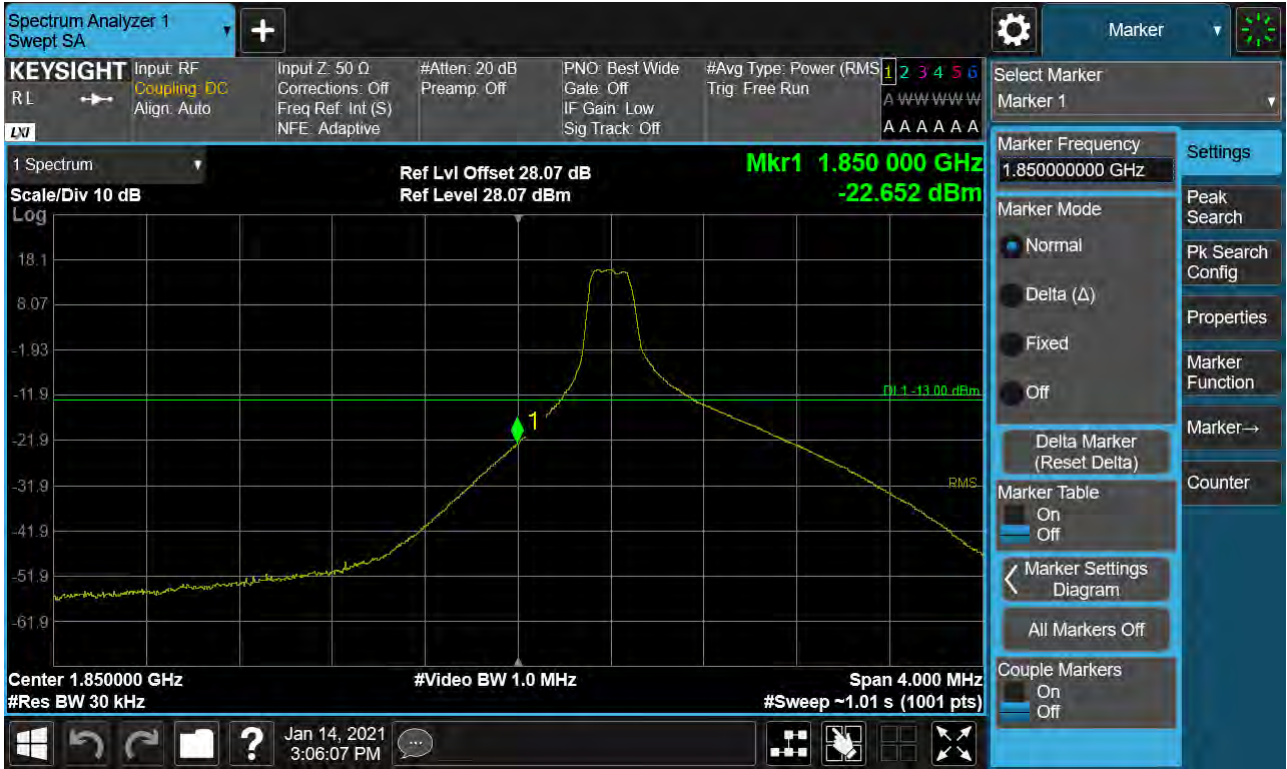
Sub6 n25. Lower Band Edge Plot (10M BW Ch.371000 BPSK_RB1_Offset 0)
