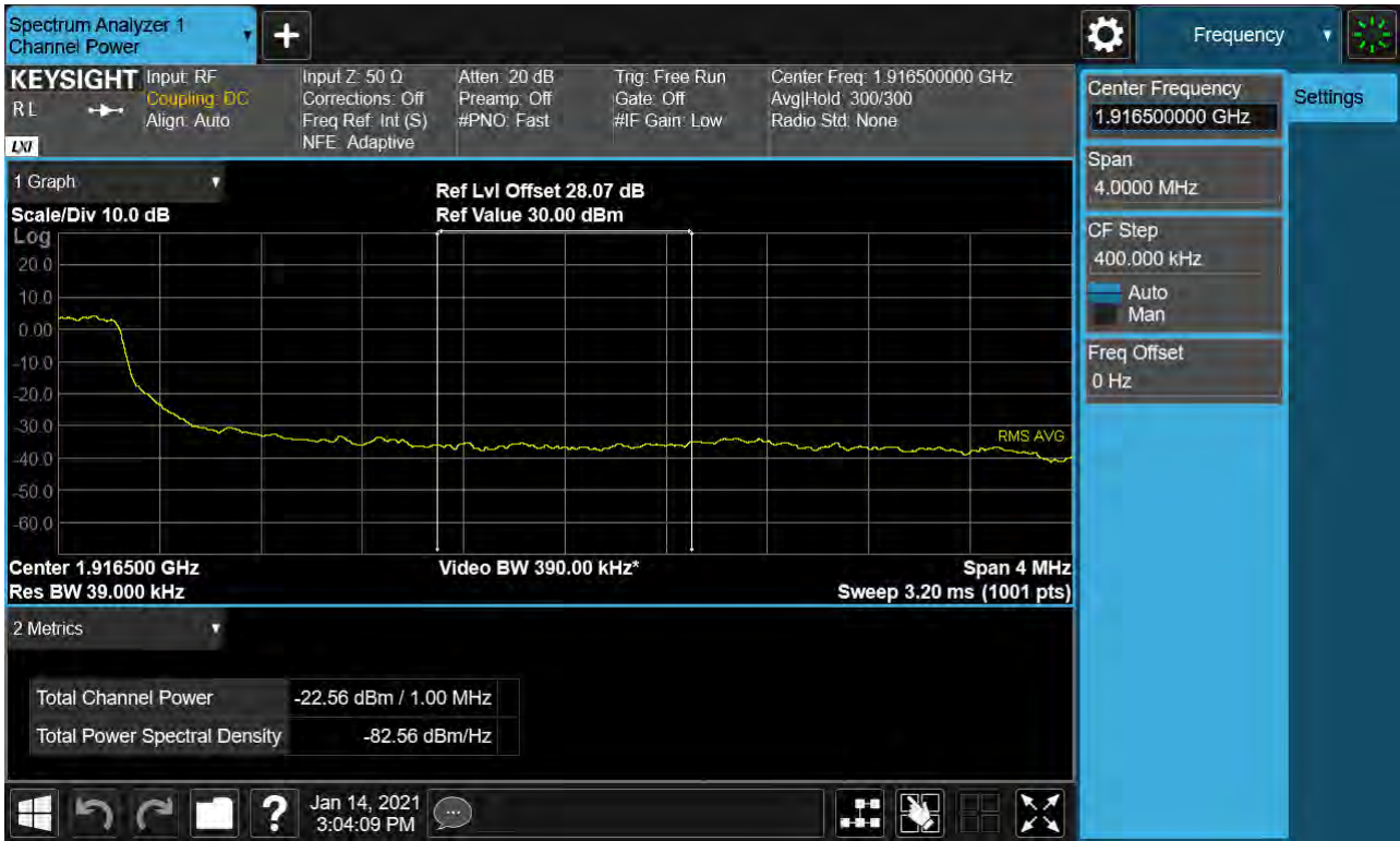
Sub6 n25. Upper Extended Band Edge Plot (5M BW Ch.382500 BPSK_RB25_0) -2
