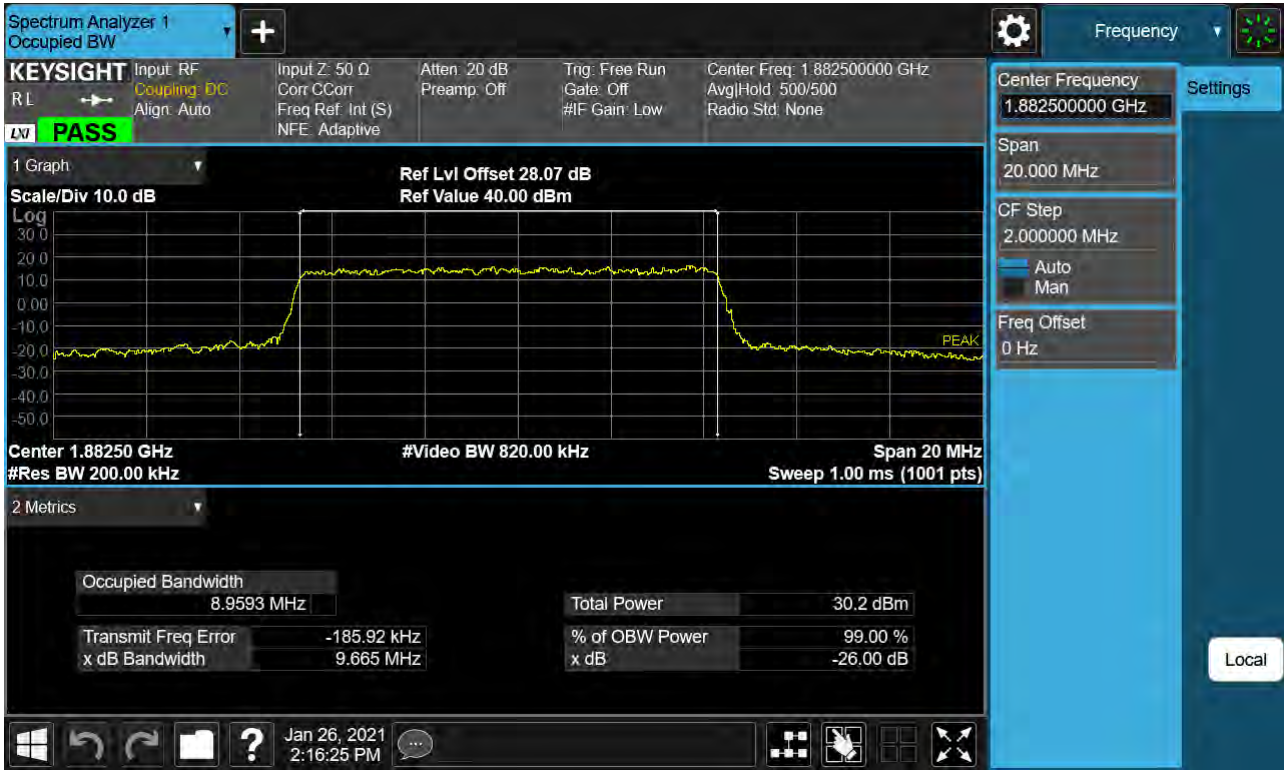
Sub6 n25. Occupied Bandwidth Plot (10M BW Ch.376500 64QAM RB 52_0)
