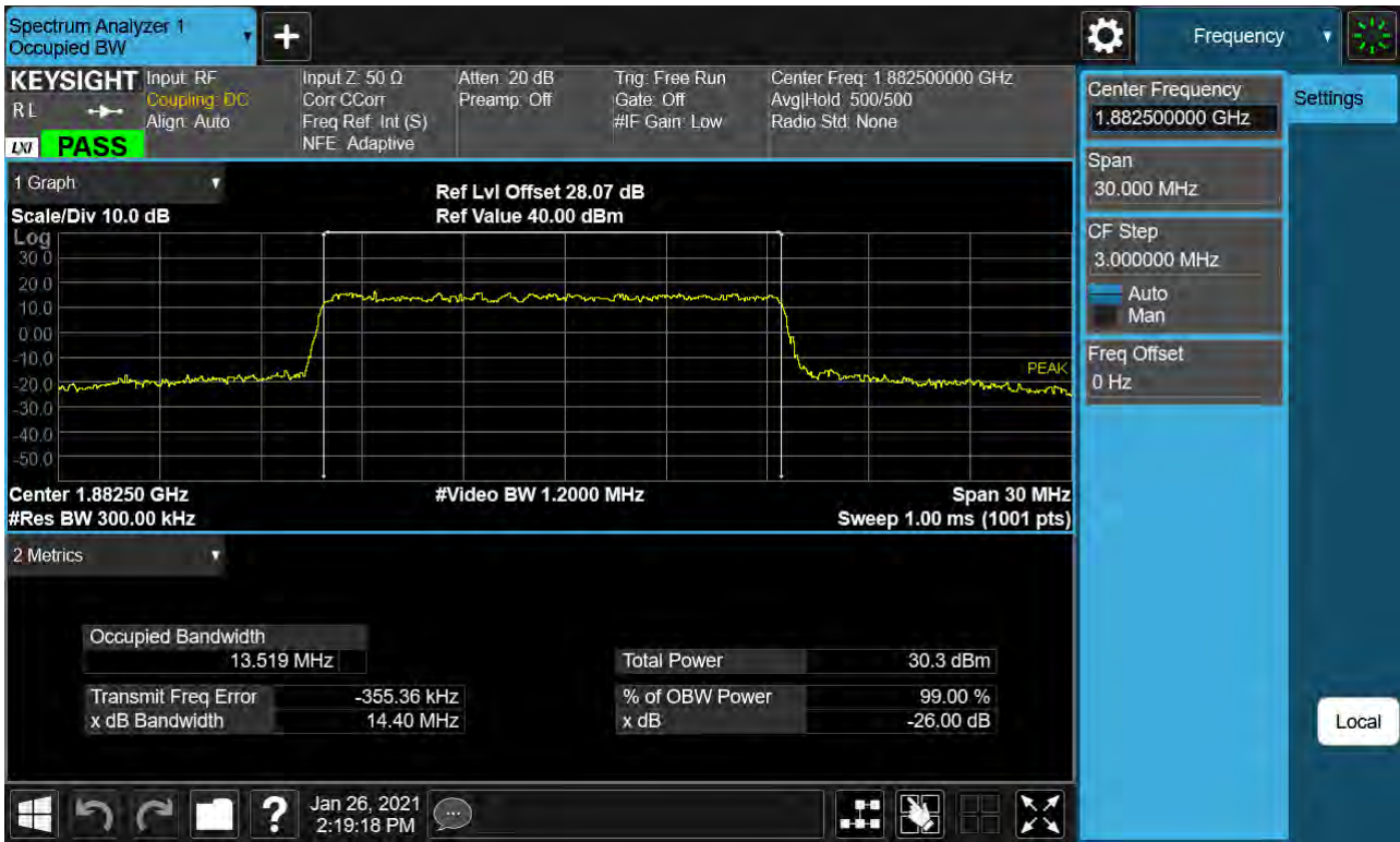
Sub6 n25. Occupied Bandwidth Plot (15M BW Ch.376500 64QAM RB 79_0)
