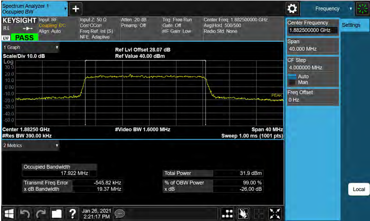
Sub6 n25. Occupied Bandwidth Plot (20M BW Ch.376500 QPSK RB 106_0)
