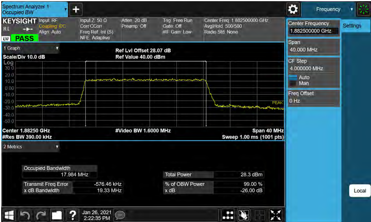
Sub6 n25. Occupied Bandwidth Plot (20M BW Ch.376500 256QAM RB 106_0)
