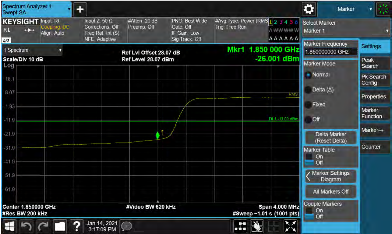
Sub6 n25. Lower Band Edge Plot (20M BW Ch.372000 BPSK_RB106_Offset 0) -1
