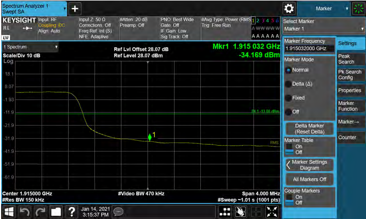
Sub6 n25. Upper Band Edge Plot (15M BW Ch.381500 BPSK_RB79_Offset 0) -1
