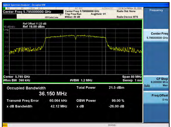
802.11n_HT40 UNII 3 BAND 26dB Bandwidth (CH 159)
