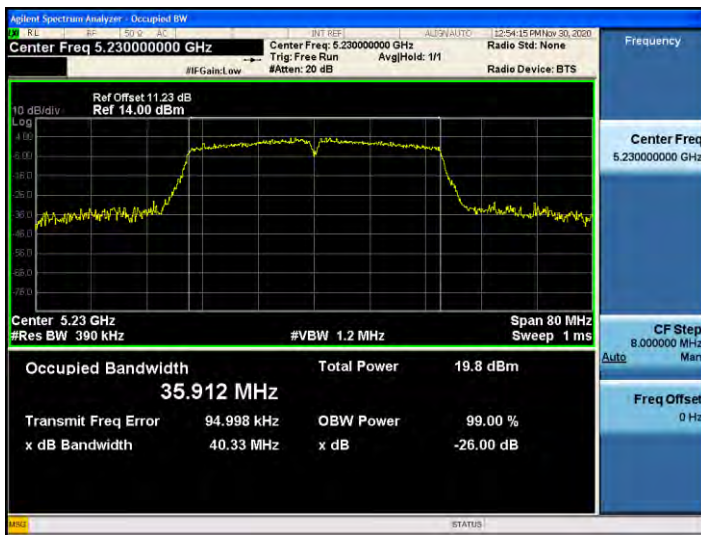
802.11ac_VHT40 UNII 2C BAND 26dB Bandwidth(CH 142)
