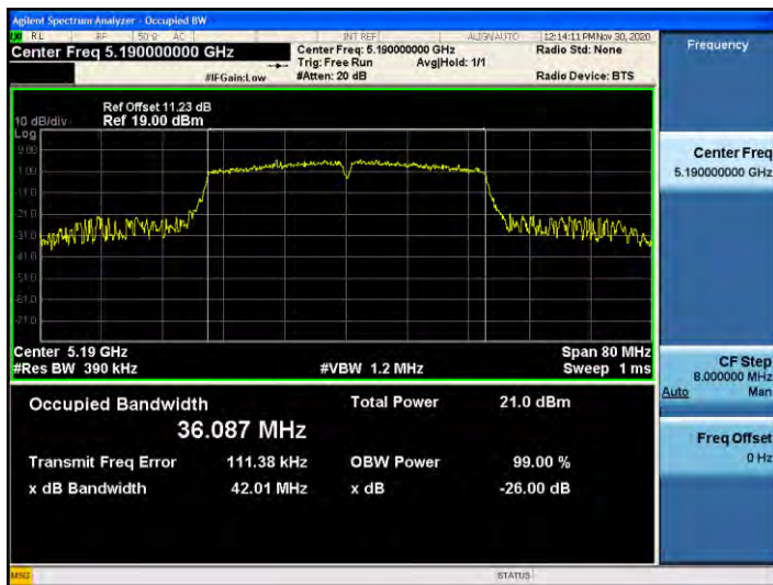
802.11n_HT40 UNII 2C BAND 26dB Bandwidth(CH 142)
