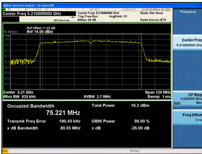
802.11ac_VHT80 UNII 2C BAND 26dB Bandwidth(CH 138)
