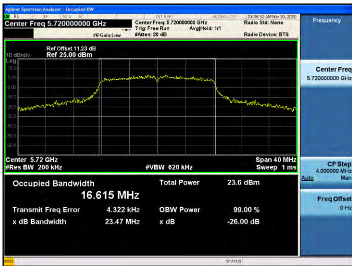
802.11a UNII 2C BAND 26dB Bandwidth (CH 144)
