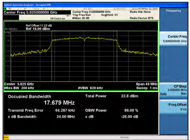
802.11n_HT20 UNII 3 BAND 26dB Bandwidth(CH 165)
