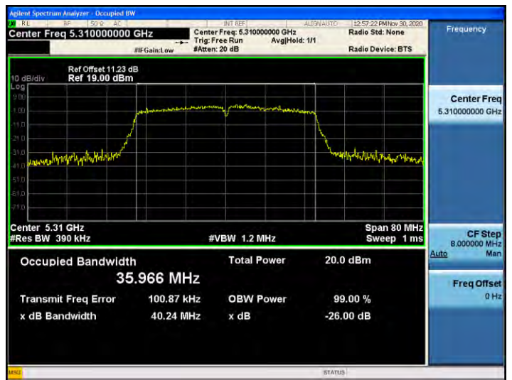
802.11ac_VHT40 UNII 3 BAND 26dB Bandwidth (CH 151)
