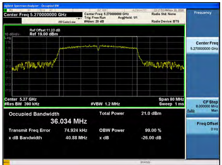
802.11n_HT40 UNII 3 BAND 26dB Bandwidth (CH 159)
