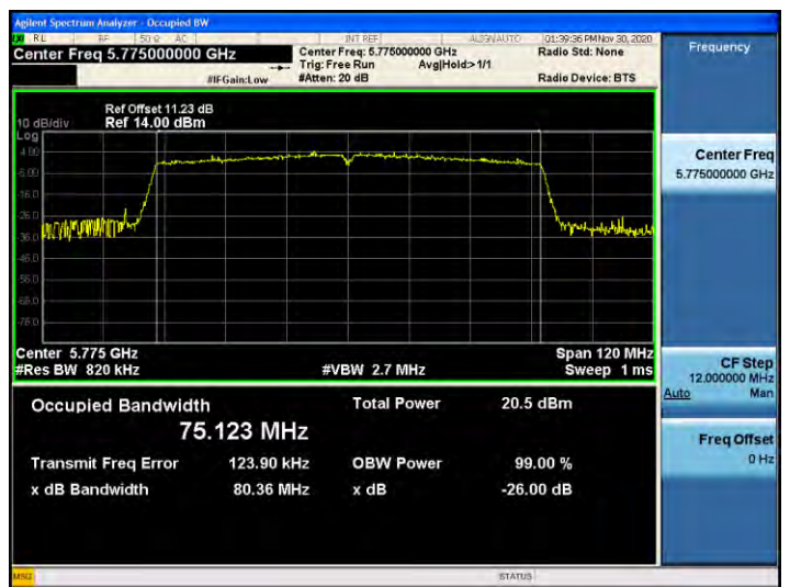
802.11ac_VHT80 UNII 3 BAND 26dB Bandwidth (CH 155)
