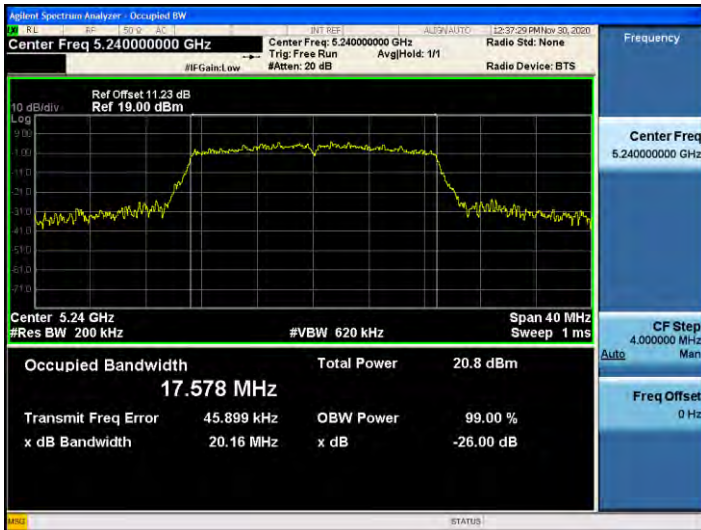
802.11ac_VHT20 UNII 2C BAND 26dB Bandwidth(CH 144)
