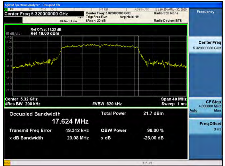
802.11n_HT20 UNII 3 BAND 26dB Bandwidth(CH 165)
