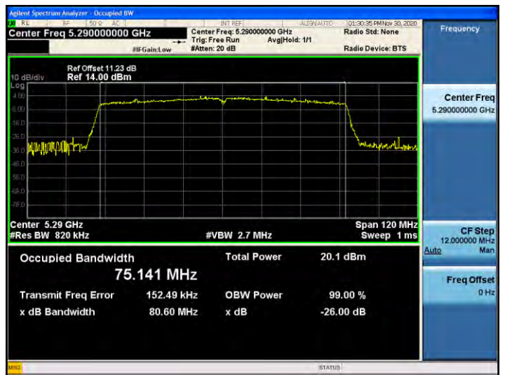
802.11ac_VHT80 UNII 3 BAND 26dB Bandwidth (CH 155)
