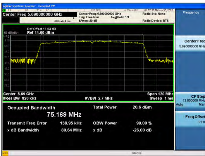
802.11ac_VHT80 UNII 2C BAND 26dB Bandwidth(CH 138)
