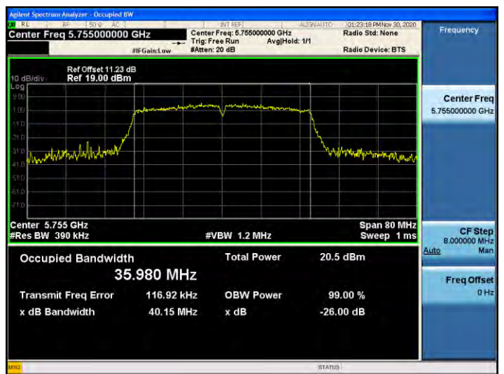
802.11ac_VHT40 UNII 3 BAND 26dB Bandwidth (CH 151)
