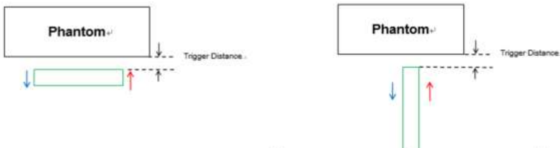
Proximity Sensor Trigger Distance Assessment KDB 616217 D04 §6.2 (Rear /Left Side)
