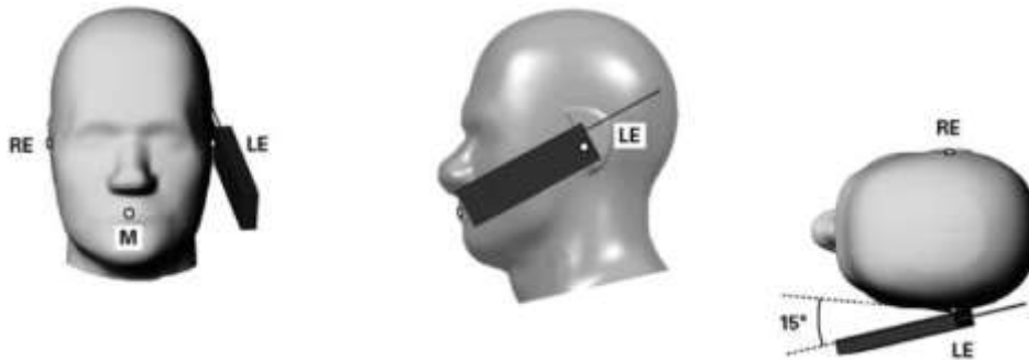
Figure 8.5. Tilt 15° position of the wireless device
