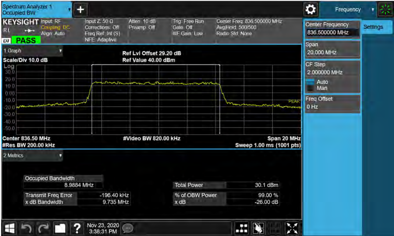
Sub6 n5. Occupied Bandwidth Plot (10M BW Ch.167300 64QAM_RB15_0)
