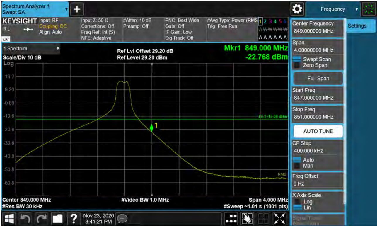
Sub6 n5. Upper Band Edge Plot (10M BW Ch.168800 BPSK_RB1_Offset 49)
