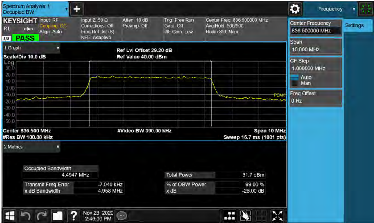
Sub6 n5. Occupied Bandwidth Plot (5M BW Ch.167300 QPSK_RB6_0)
