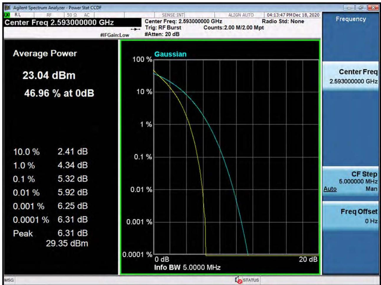
BAND 41. PAR Plot (5M BW\_Ch.40620\_16QAM\_RB25\_0)
