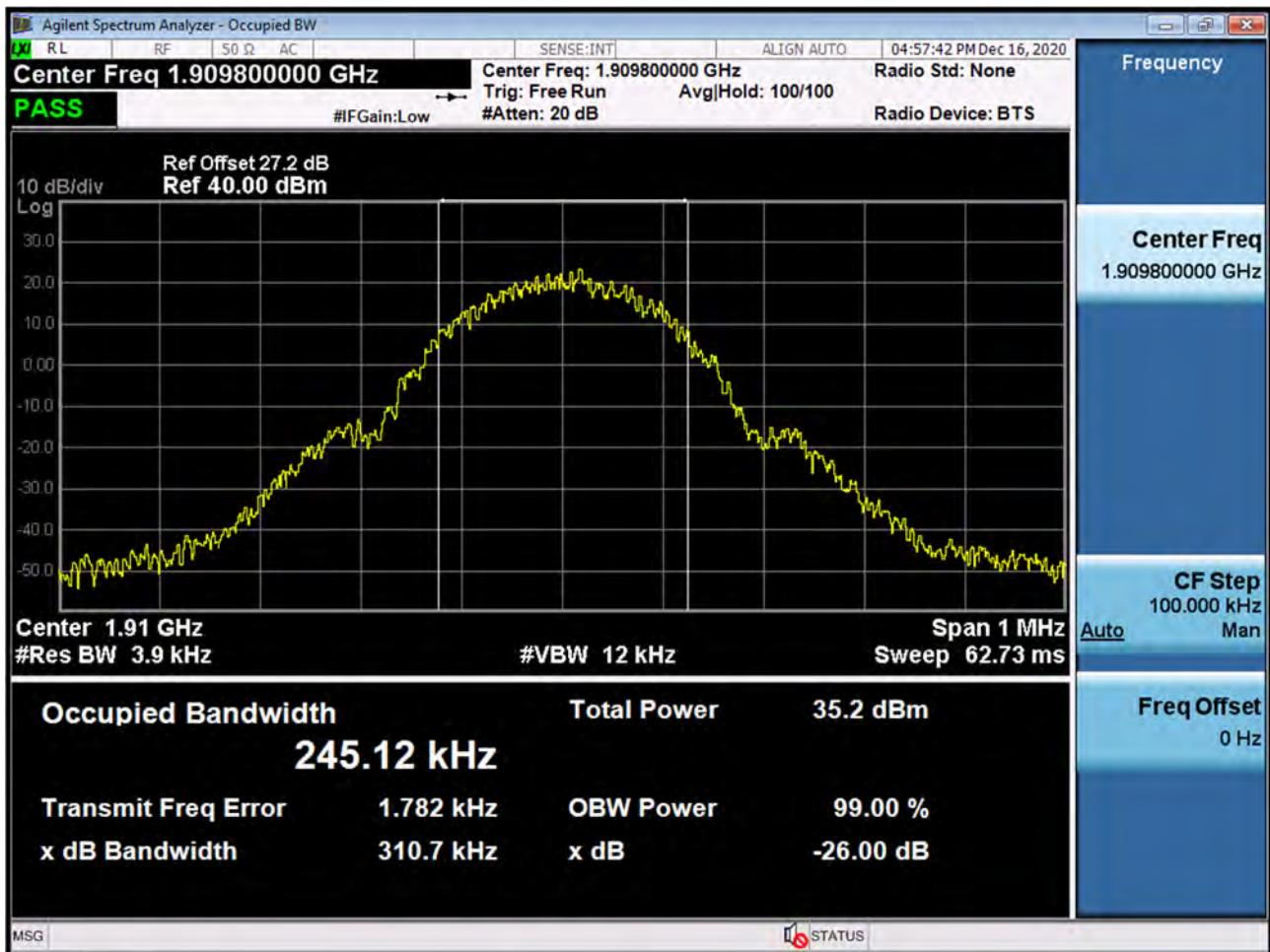
■ GSM1900 EDGE (512 CH.) Occupied Bandwidth
