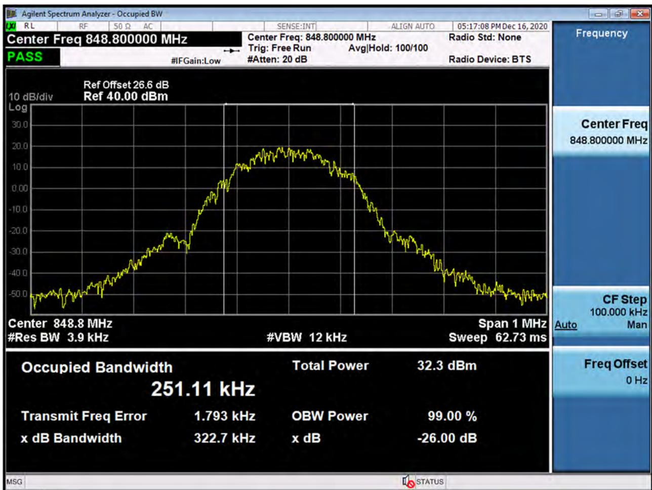
■ GSM1900 MODE (512 CH.) Occupied Bandwidth
