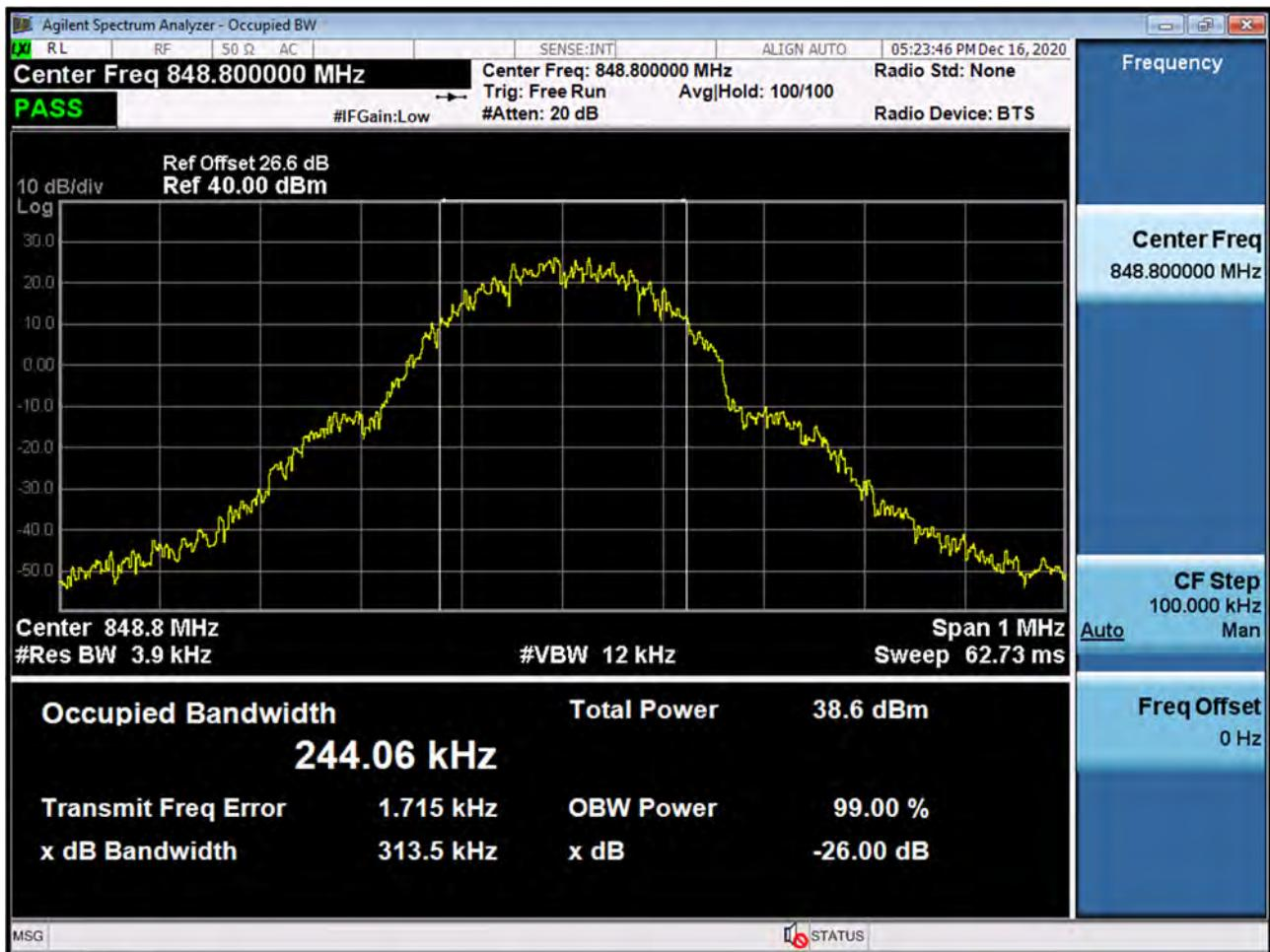
■ GSM850 EDGE (251 CH.) Occupied Bandwidth
