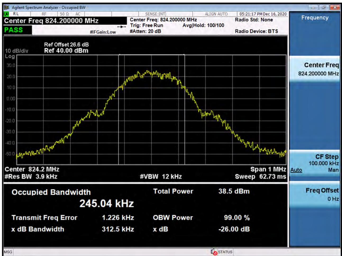
■ GSM850 MODE (190 CH.) Occupied Bandwidth
