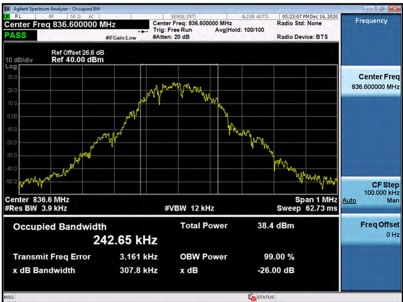
■ GSM850 MODE (251 CH.) Occupied Bandwidth
