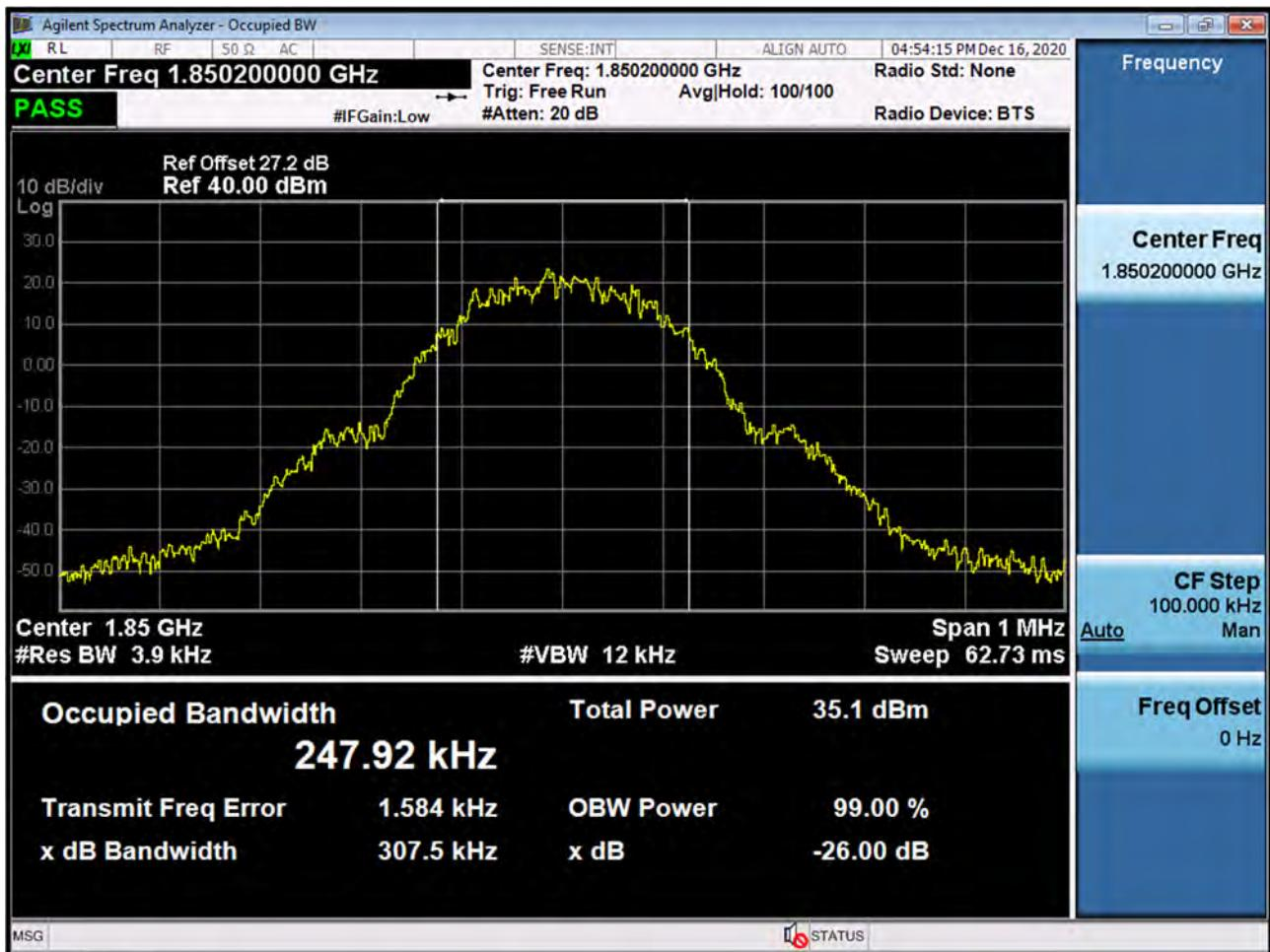
■ GSM1900 MODE (661 CH.) Occupied Bandwidth
