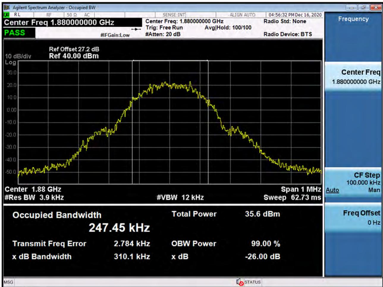
■ GSM1900 MODE (810 CH.) Occupied Bandwidth
